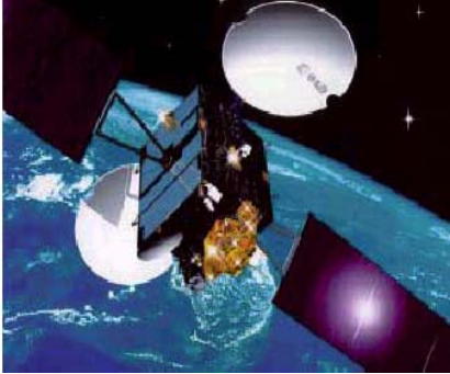
Fig. 2 Typical spacecraft structure with a plate-like behavior such as antenna, solar panel and a box as main spacecraft structure
