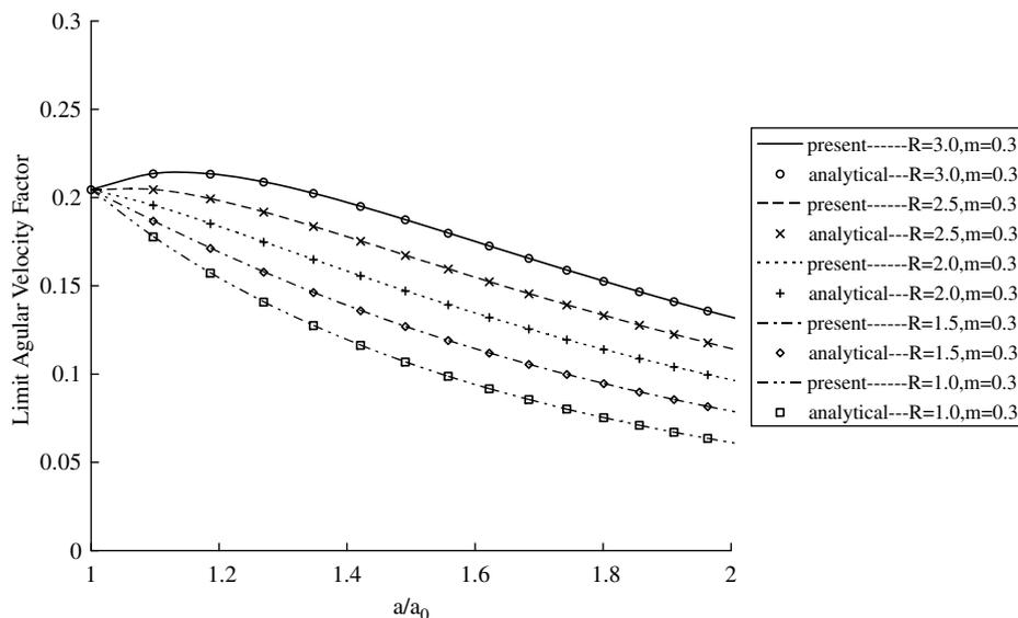
Fig. 5. Effect of yield strength ratio  $R = \sigma_\infty/\sigma_0$  on the normalized plastic limit angular velocity factor  $\rho\omega^2 b_0^2/\sigma_0$  with strain-rate sensitivity  $m = 0.3$ .
