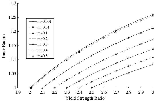
Fig. 6. Effect of strain-rate sensitivity  $m$  and yield strength ratio  $R = \sigma_\infty/\sigma_0$  on the onset of instability in terms of the inner radius  $a/a_0$ .
