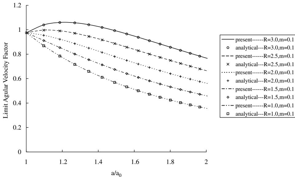
Fig. 4. Effect of yield strength ratio  $R = \sigma_\infty/\sigma_0$  on the normalized plastic limit angular velocity factor  $\rho\omega^2 b_0^2/\sigma_0$  with strain-rate sensitivity  $m = 0.1$ .
