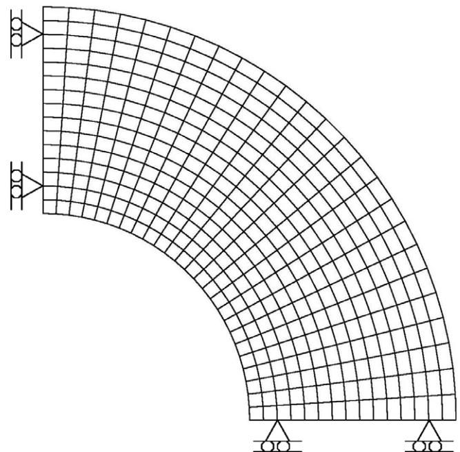
Fig. 1. Finite-element model of a rotating hollow cylinder.
