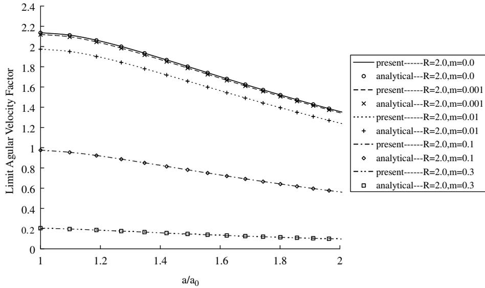
Fig. 2. Effect of strain-rate sensitivity  $m$  on the normalized plastic limit angular velocity factor  $\rho\omega^2 b_0^2/\sigma_0$  with yield strength ratio  $R = \sigma_\infty/\sigma_0 = 2$ .
