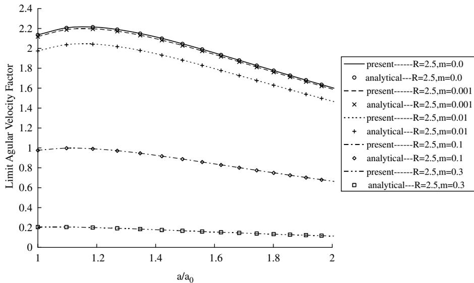
Fig. 3. Effect of strain-rate sensitivity  $m$  on the normalized plastic limit angular velocity factor  $\rho\omega^2 b_0^2/\sigma_0$  with yield strength ratio  $R = \sigma_\infty/\sigma_0 = 2.5$ .
