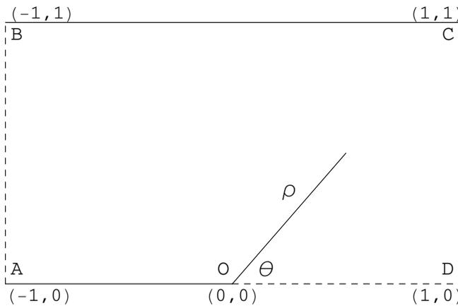
Figure 5: The cracked beam problem. The solid line corresponds to the Dirichlet boundary condition and the dashed line denotes Neumann's condition. Here  $(\rho, \theta)$  is the local polar coordinate system with the origin at the singular point.
