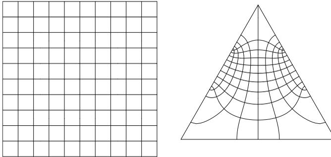
Figure 6: The conformal map obtained by the combination of the analytic map of the unit square onto the circle and the numerical conformal map of the circle onto the equilateral triangle.
