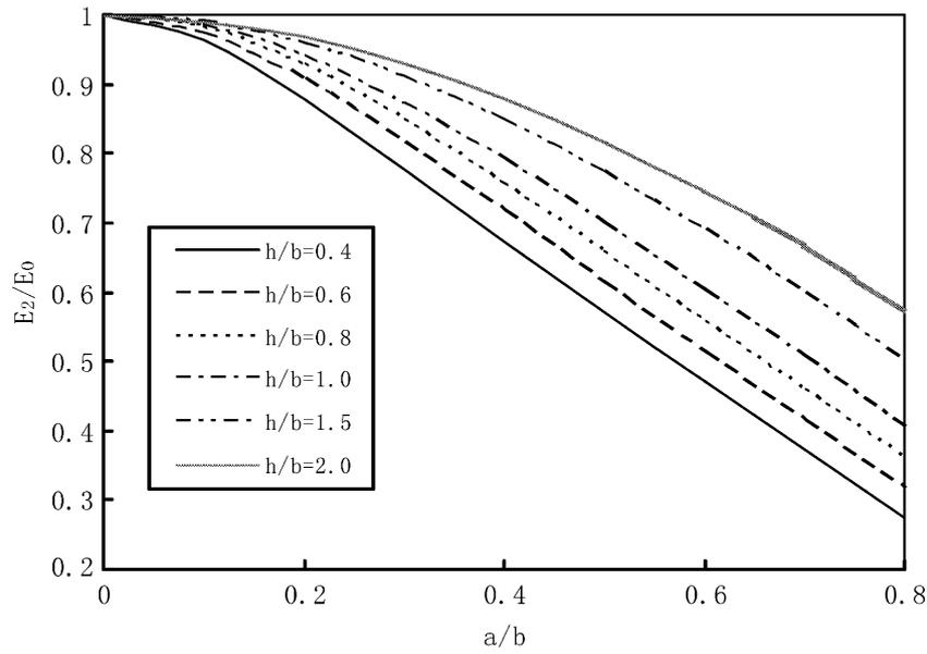
Figure 6. Normalized effective elastic modulus  $E_2/E_0$  for an infinite domain containing doubly periodic array of cracks.
