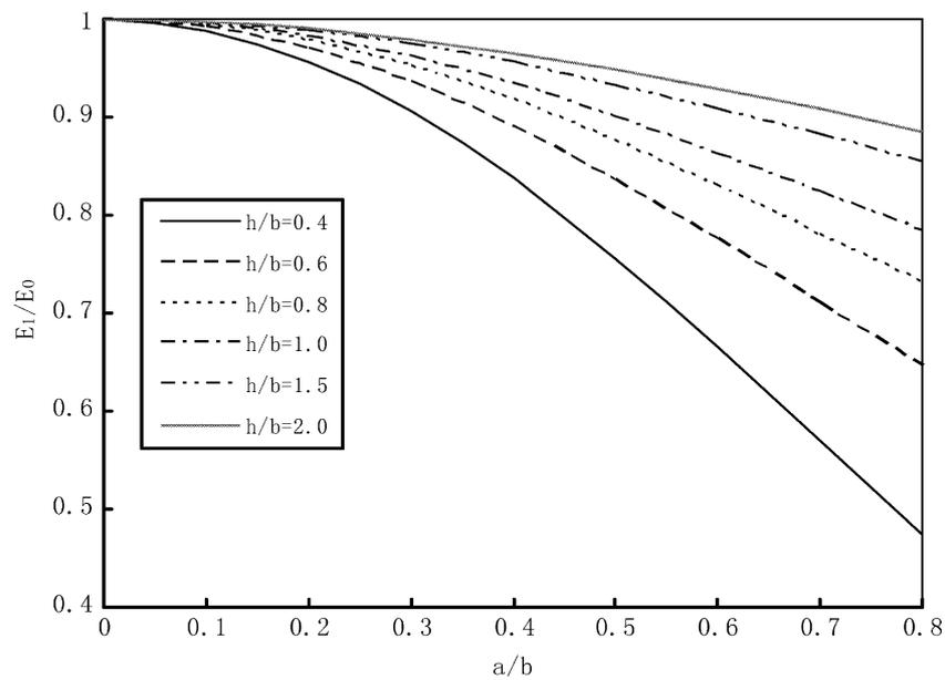
Figure 11. Normalized effective elastic modulus  $E_1/E_0$  for an infinite domain containing doubly periodic array of rigid-line inclusions.
