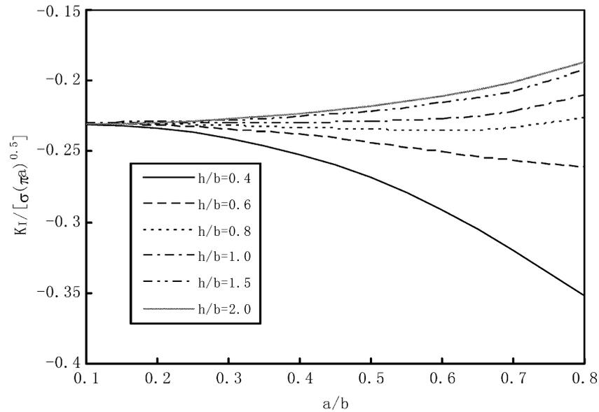
Figure 10. Normalized stress intensity factor  $K_I / [\sigma \sqrt{\pi a}]^{0.5}$  for an infinite domain containing doubly periodic array of rigid-line inclusions subjected to a remote tension loading  $\sigma$  along  $x_2$ -direction.
