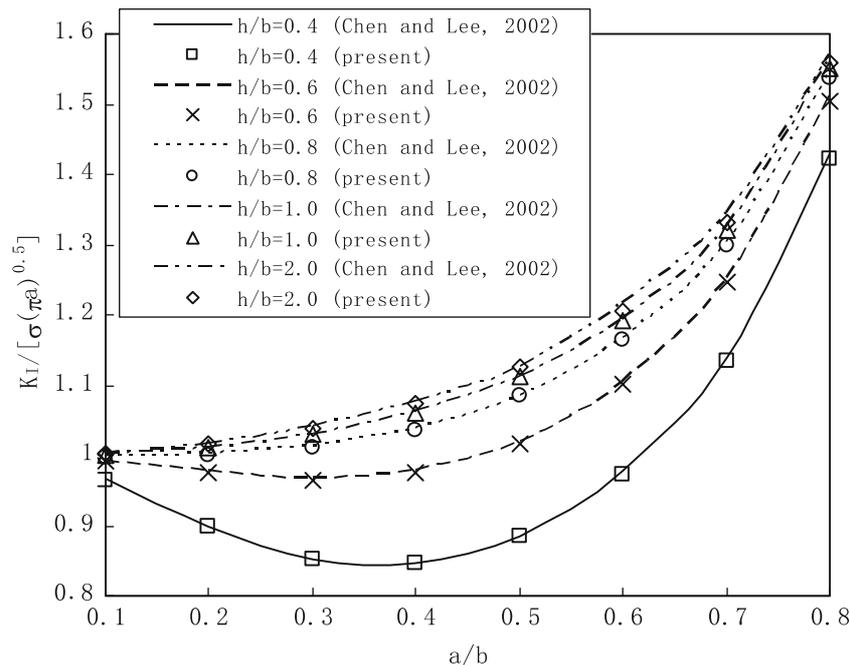
Figure 4. Normalized stress intensity factor  $K_I/[\sigma\sqrt{\pi a}]$  for an infinite domain containing doubly periodic array of cracks subjected to a remote tension loading  $\sigma$  along  $x_2$ -direction.
