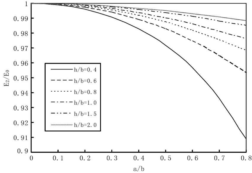
Figure 12. Normalized effective elastic modulus  $E_2/E_0$  for an infinite domain containing doubly periodic array of rigid-line inclusions.
