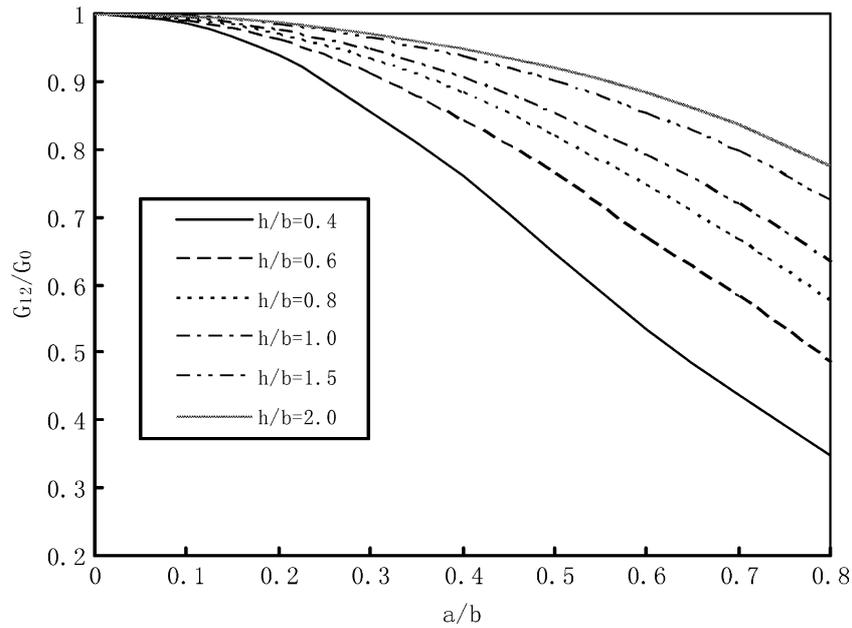
Figure 7. Normalized effective shear modulus  $G_{12}/G_0$  for an infinite domain containing doubly periodic array of cracks.
