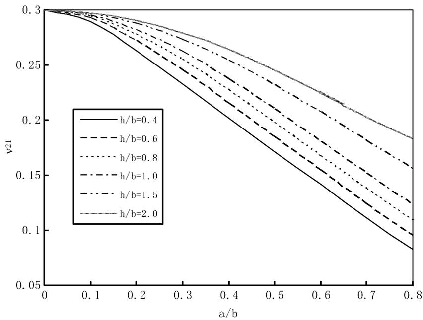
Figure 8. Effective Poisson's ratio  $v_{21}$  for an infinite domain containing doubly periodic array of cracks.
