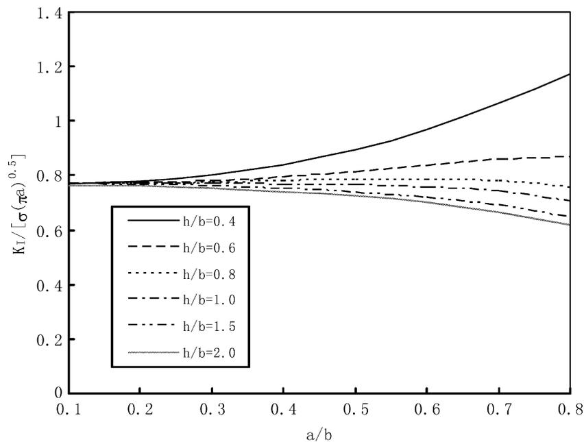
Figure 9. Normalized stress intensity factor  $K_I / [\sigma \sqrt{\pi a}]$  for an infinite domain containing doubly periodic array of rigid-line inclusions subjected to a remote tension loading  $\sigma$  along  $x_1$ -direction.
