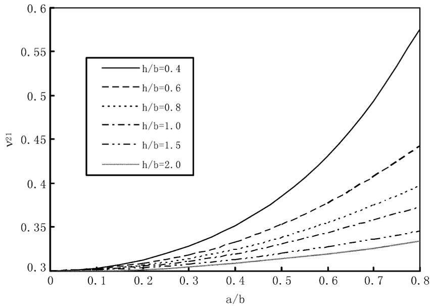
Figure 13. Effective Poisson's ratio  $\nu_{21}$  for an infinite domain containing doubly periodic array of rigid-line inclusions.
