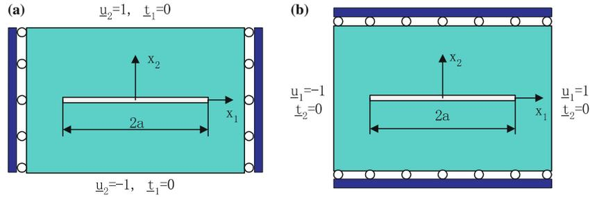
Figure 2. Sub-problems from the boundary value problem as shown in Figure 1b1. The boundary condition of sub-problems b2–b5 is the same as sub-problem (b1).
