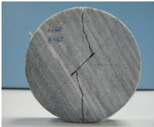
Figure 23. Photograph of specimen EM-4 after failure ( $\psi = 60^\circ$  and  $\beta = 45^\circ$ ).
