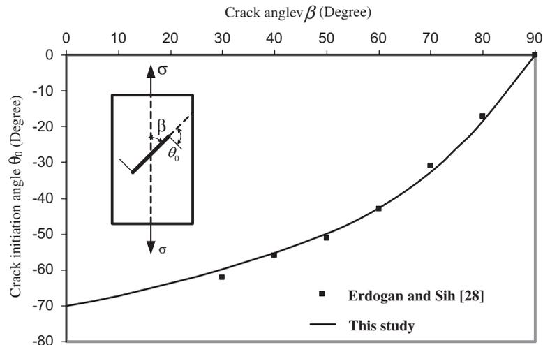
Figure 12. Variation of crack initiation angle  $\theta_0$  with the crack angle  $\beta$ . Plexiglass plate subjected to uniaxial tension.
