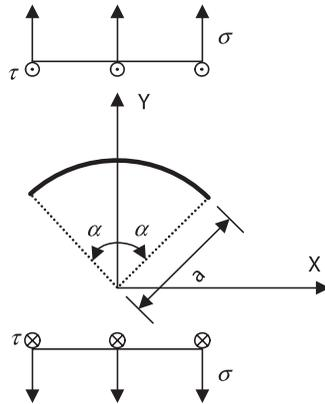
Figure 9. A curved crack under a far-field tensile stress  $\sigma$  and out-of-plane shear stress  $\tau$ .
