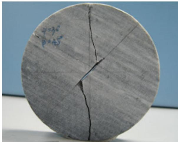
Figure 19. Photograph of specimen CM-4 after failure ( $\psi = 30^\circ$  and  $\beta = 45^\circ$ ).
