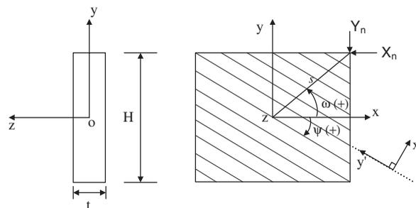
Figure 2. The definition of coordinate system on anisotropic plate.
