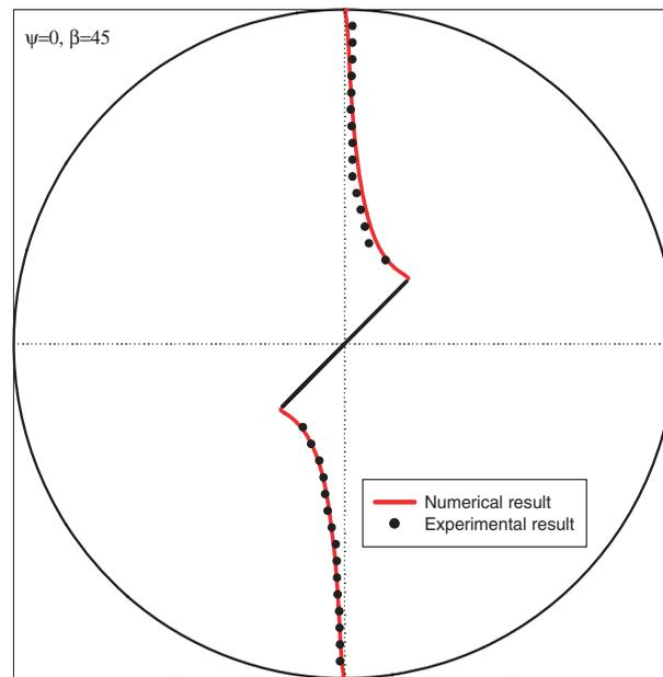
Figure 18. Propagation of a crack at the center of a CSTBD specimen with  $\psi = 0^\circ$  and  $\beta = 45^\circ$ . Comparison between experimental observations and numerical predictions for specimen AM-4.
