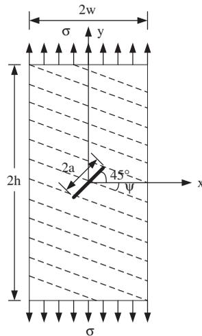
Figure 11. An anisotropic rectangular plate with a central crack inclined 45° under uniform tensile stress  $\sigma$ .
