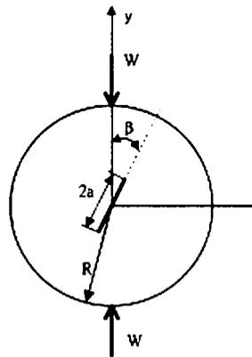
Figure 8. The geometry of cracked Brazilian disc.
