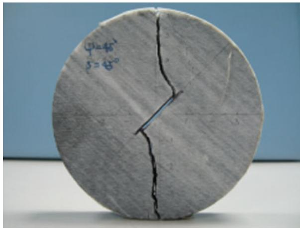
Figure 21. Photograph of specimen DM-4 after failure ( $\psi = 45^\circ$  and  $\beta = 45^\circ$ ).
