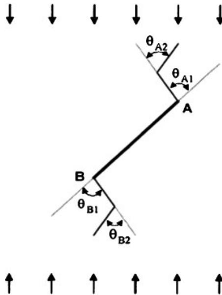
Figure 6. Process of crack propagation by increasing the number of linear elements.
