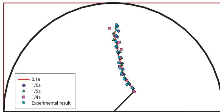
Figure 5. Crack propagation path simulation with different incremental lengths for half-CSTBD specimen ( $\psi = 30^\circ$ ,  $\beta = 45^\circ$ ).
