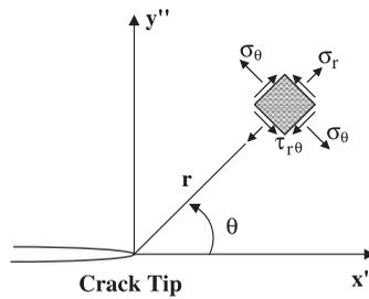
Figure 4. Crack tip coordinate system and stress components.
