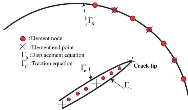
Figure 3. Geometry of a two-dimensional cracked domain.
