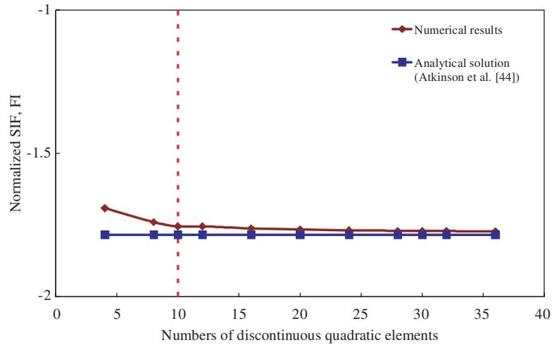
Figure 7. Variation of normalized SIF of mode I with different elements of crack surface.
