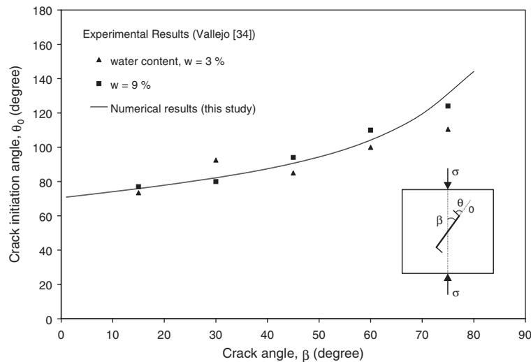
Figure 13. Variation of crack initiation angle  $\theta_0$  with the crack angle  $\beta$ . Prismatic sample of kaolinite clay subjected to uniaxial compression.
