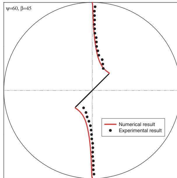
Figure 24. Propagation of a crack at the center of a CSTBD specimen with  $\psi = 60^\circ$  and  $\beta = 45^\circ$ . Comparison between experimental observations and numerical predictions for specimen EM-4.
