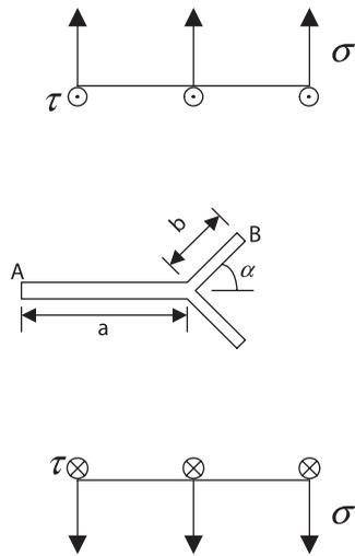
Figure 10. Branched crack under a far-field tensile stress  $\sigma$  and out-of-plane shear stress  $\tau$ .
