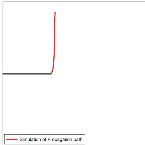
Figure 16. Crack propagation path and normalized SIFs of the cracked plate initially under pure mode II loading.
