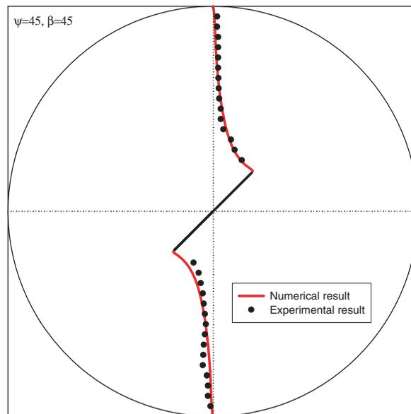
Figure 22. Propagation of a crack at the center of a CSTBD specimen with  $\psi = 45^\circ$  and  $\beta = 45^\circ$ . Comparison between experimental observations and numerical predictions for specimen DM-4.
