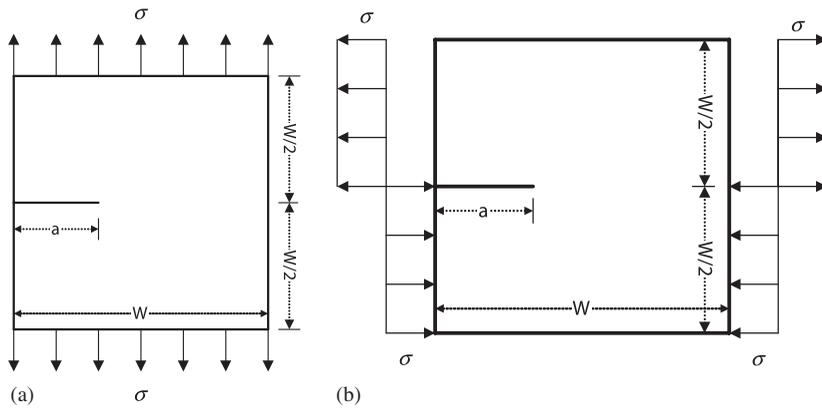
Figure 14. Square plate with a straight edge crack under pure mode I and mode II.
