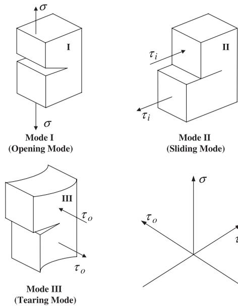
Figure 1. Basic modes of fracture.
