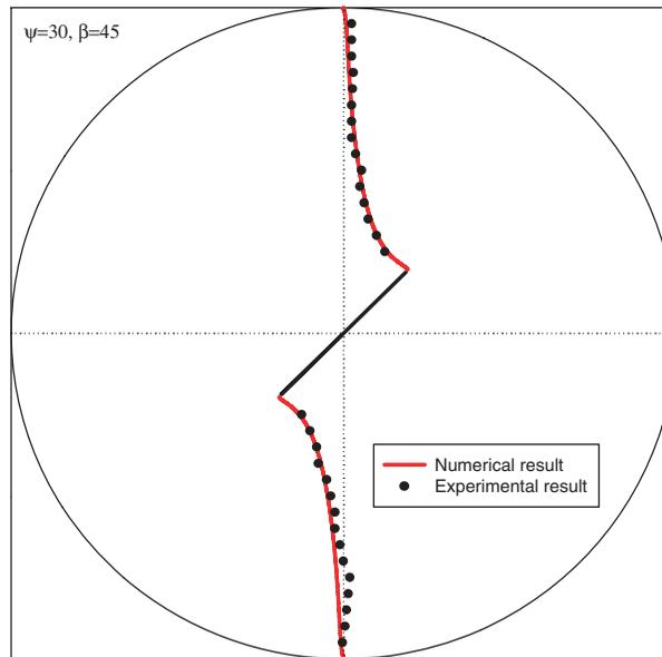
Figure 20. Propagation of a crack at the center of a CSTBD specimen with  $\psi = 30^\circ$  and  $\beta = 45^\circ$ . Comparison between experimental observations and numerical predictions for specimen CM-4.
