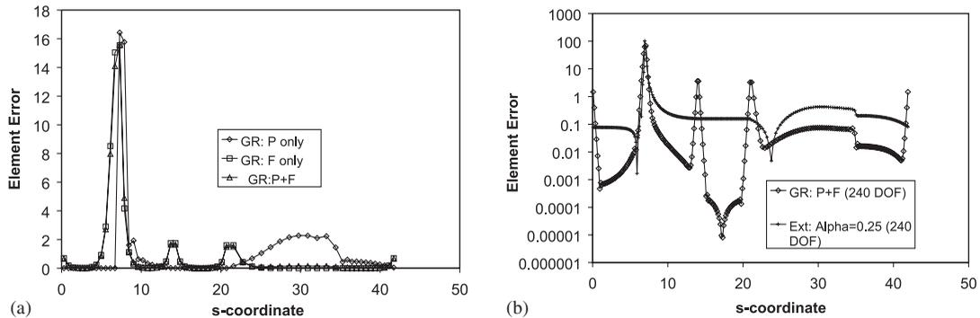
Figure 4. Motz problem: (a) Influence of the individual contributions of potential only (GR:P) and flux only (GR:F) for the gradient recovery (GR:P+F) error estimator for the 60 elements mesh; (b) comparison between gradient recovery (GR:P+F) and External ( $\alpha=0.25$ ) error estimators for the 240 elements mesh.
