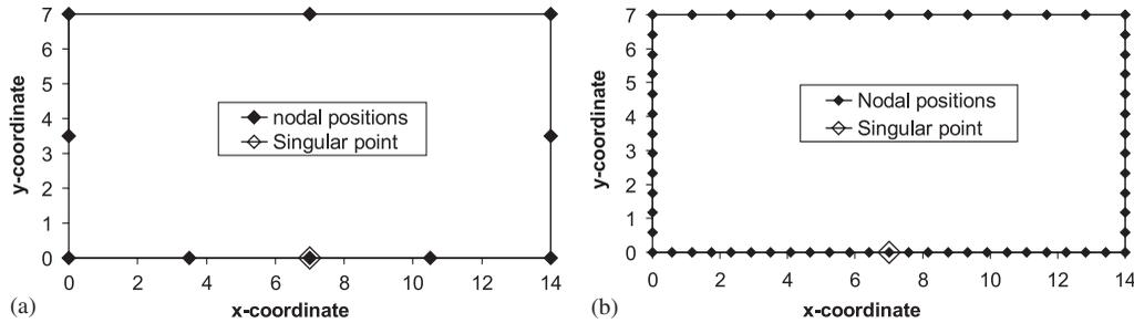
Figure 2. Meshes for the Motz problem: (a) coarse mesh: 10 elements; and (b) a finer mesh: 60 elements.
