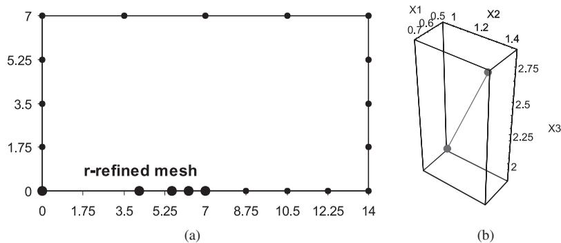
Figure 12. Solution of the optimization procedure. Minimizer is  $\{x_1, x_2, x_3\}_* = \{0.71, 1.42, 2.84\}$ : (a) smaller elements are obtained near the singular point; and (b) solution is obtained in one step only starting from the point  $\{x_1, x_2, x_3\}_0 = \{0.47, 0.93, 1.87\}$ , corresponding to the working set  $W = \{g_2, g_4, g_6\}$ .
