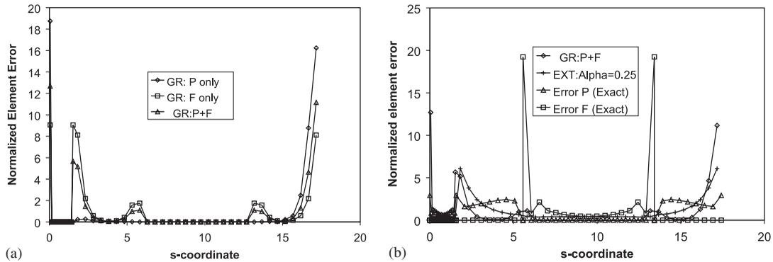
Figure 8. Pipe problem: (a) influence of the individual contributions of potential only (GR:P) and flux only (GR:F) for the gradient recovery (GR:P+F) error estimator for the 48 elements mesh; and (b) comparison between gradient recovery (GR:P+F) and External ( $\alpha=0.25$ ) error estimators for the 24 elements mesh. Also included the errors with respect to the known exact boundary solution.
