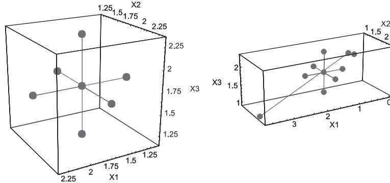
Figure 11. Position of the points in the adapted partial central design of experiments (DOE) approach.
