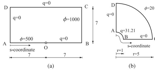
Figure 1. Numerical examples: (a) the Motz problem: a singularity is created at point  $O$  by the mixed boundary conditions; and (b) axisymmetric heat conduction in a pipe. One-quarter of the pipe cross-section is modelled.
