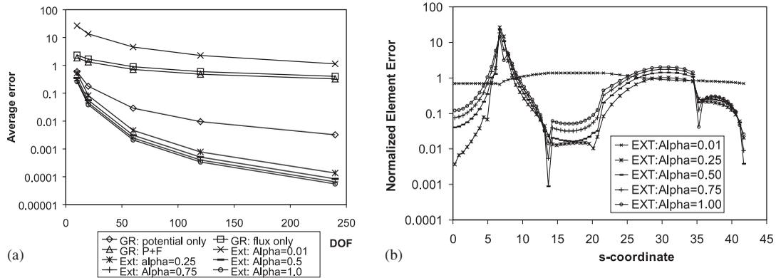
Figure 3. Motz problem: (a) average (global) error estimators for the gradient recovery (GR) procedure and for the external domain (Ext) approach for various values of  $\alpha$ ; and (b) influence of the position of the external point for the 60 elements mesh. Plotted error results for various values of  $\alpha$ .
