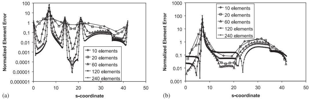
Figure 5. Motz problem: influence of mesh refinement for: (a) the gradient recovery (GR) error estimator with potential and flux combined; and (b) the external domain (Ext) error estimator with  $\alpha=0.25$ .
