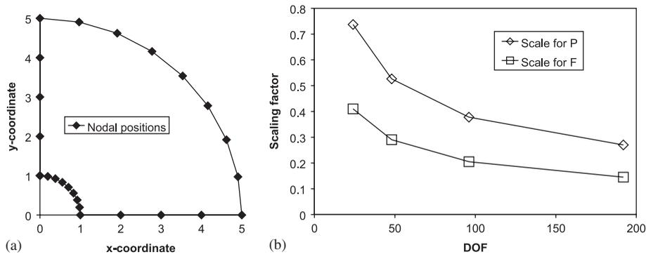
Figure 6. Pipe problem: (a) coarse mesh: 24 elements; and (b) scaling factors for the gradient recovery (GR:P+F) error estimator. Individual contributions of the potential (P) only and of the flux (F) only are scaled before combined to give the GR:P+F error estimator.
