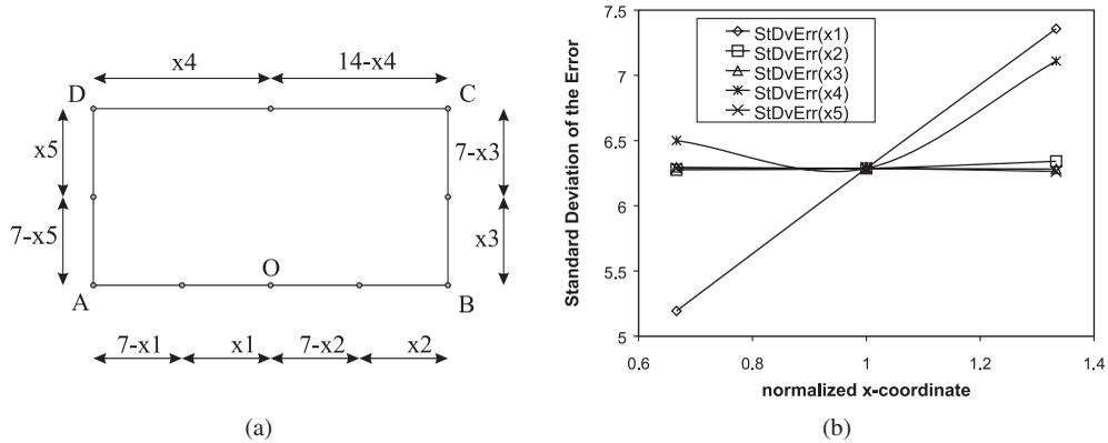
Figure 9. Coarse mesh: (a) the variables  $x_1, x_2, x_3, x_4$  and  $x_5$  correspond to the position of the interior nodes in each linear segment  $AO, OB, BC, CD$  and  $DA$ . Position of interior nodes can vary separately; and (b) sensitivity of the standard deviation of the element error with element size variations in different regions of the boundary. Horizontal axis is a normalized  $x$ -co-ordinate given by  $x_i/(x_i)_{(initial)}$ , for  $i = 1, 2, 3, 4, 5$ .
