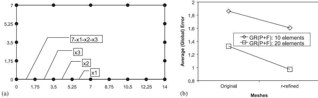
Figure 10. (a) Finer mesh: The variables  $x_1, x_2$  and  $x_3$  correspond to the position of the 3 nodes internal to the linear segment  $AO$ . Position of these nodes can vary separately; and (b) influence of  $r$ -refinement for the coarse and fine meshes, measured by the average (global) gradient recovery error estimator with potential and flux combined (GR : P+F).
