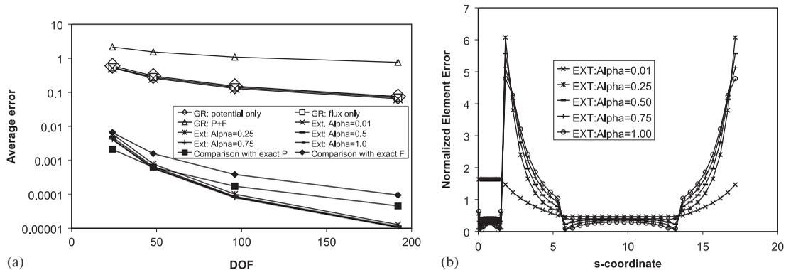
Figure 7. Pipe problem: (a) average (global) error estimators for the gradient recovery (GR) procedure and for the external domain (Ext) approach for various values of  $\alpha$ . Also included the errors with respect to the known exact boundary solution; and (b) influence of the position of the external point for the 48 elements mesh. Plotted error results for various values of  $\alpha$ .
