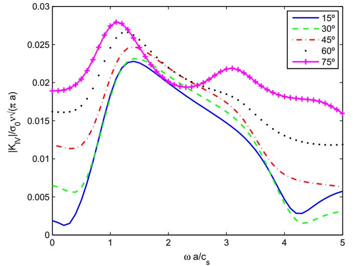
**Fig. 12.** L-wave scattering by a curved crack:  $K_{IV}$  vs. frequency for different arch angles  $\alpha$ .
