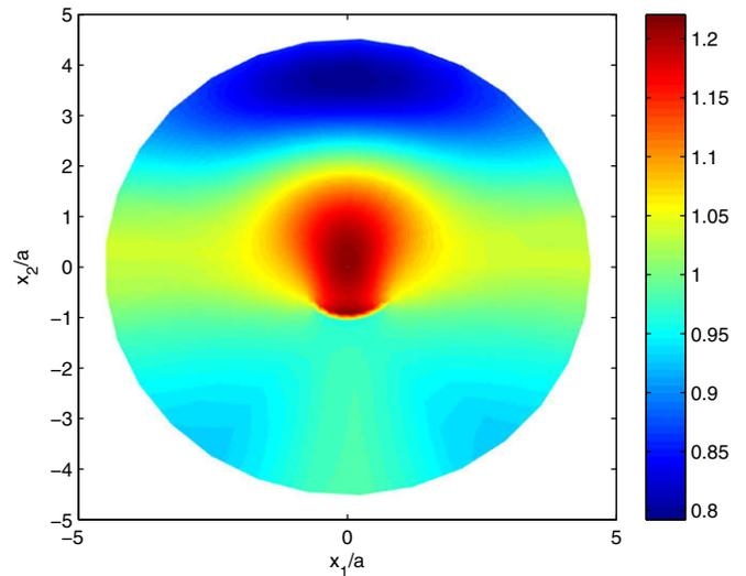
Fig. 17. L-wave scattering by a curved arch crack ( $\alpha = 45$ ): magnetic potential amplitude  $\phi/\phi_0$  at frequency  $\omega a/c_s = 0.8$ .
