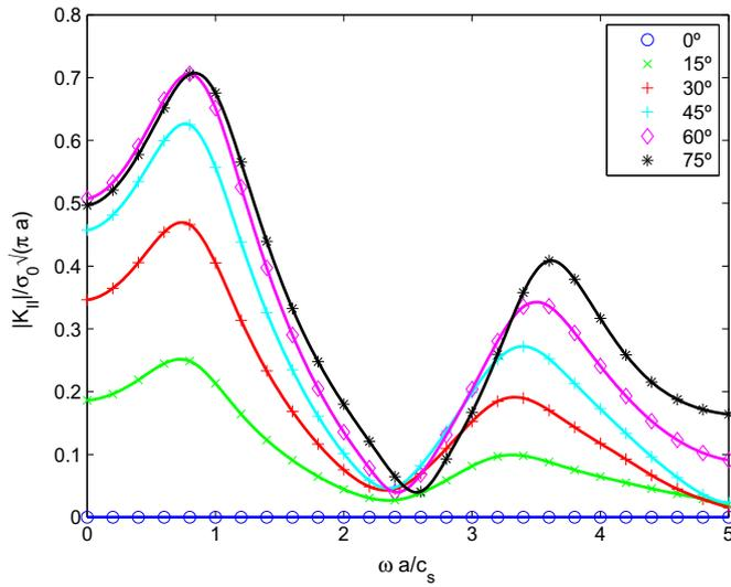
Fig. 7. L-wave scattering by a branched crack:  $K_{II}$  at branch tip vs. frequency for different branch angles  $\beta$ .
