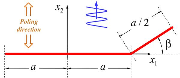
Fig. 4. Branched crack under impinging L-waves.
