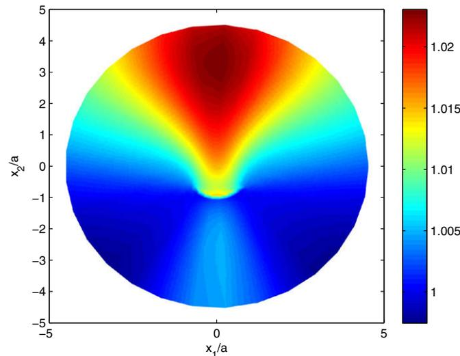
Fig. 15. L-wave scattering by a curved arch crack ( $\alpha = 45$ ): magnetic potential amplitude  $\phi/\phi_0$  at frequency  $\omega a/c_s = 0.3$ .
