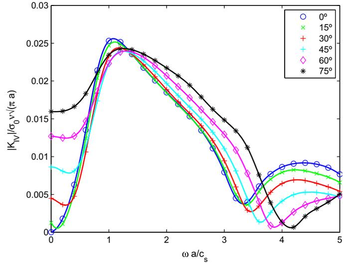
Fig. 8. L-wave scattering by a branched crack:  $K_{IV}$  at branch tip vs. frequency for different branch angles  $\beta$ .
