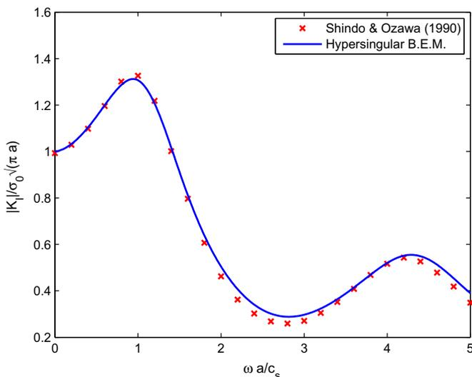
Fig. 3. Validation of the results: L-wave scattering by a Griffith crack in PZT-6B,  $K_I$  vs frequency.
