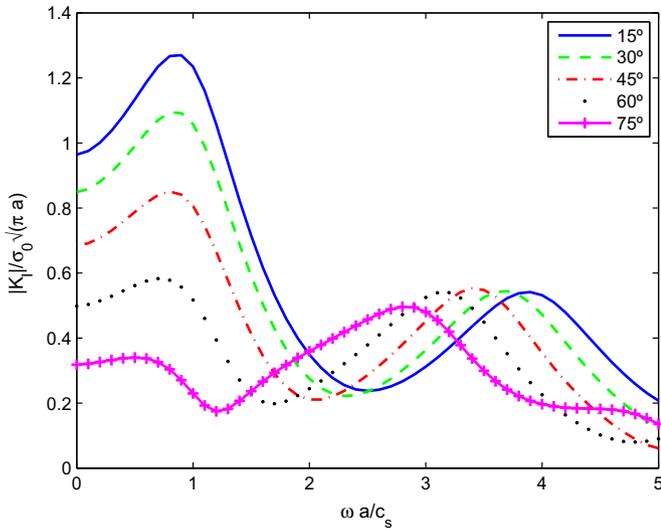
**Fig. 10.** L-wave scattering by a curved crack:  $K_I$  vs. frequency for different arch angles  $\alpha$ .
