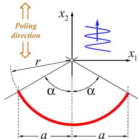
Fig. 5. Circular arch crack under impinging L-waves.
