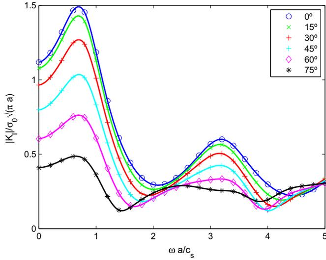
Fig. 6. L-wave scattering by a branched crack:  $K_I$  at branch tip vs. frequency for different branch angles  $\beta$ .
