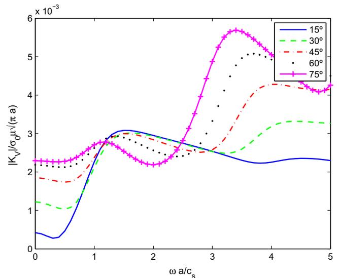
**Fig. 13.** L-wave scattering by a curved crack:  $K_V$  vs. frequency for different arch angles  $\alpha$ .
