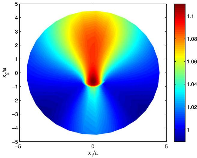
Fig. 14. L-wave scattering by a curved arch crack ( $\alpha = 45$ ): vertical displacements amplitude  $u_2/u_0$  at frequency  $\omega a/c_s = 0.3$ .
