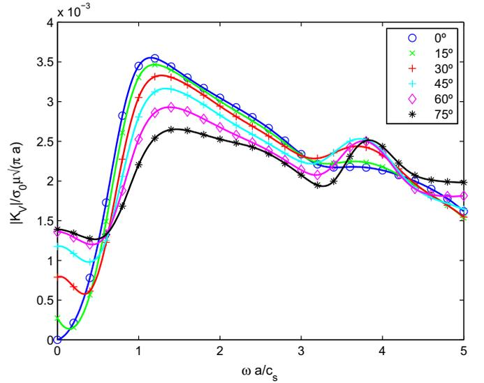
Fig. 9. L-wave scattering by a branched crack:  $K_V$  at branch tip vs. frequency for different branch angles  $\beta$ .
