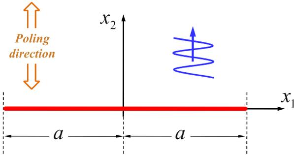
Fig. 2. Wave scattering by a Griffith crack in a PZT-6B piezoelectric solid.
