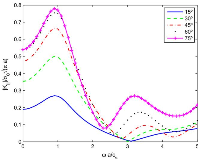
**Fig. 11.** L-wave scattering by a curved crack:  $K_{II}$  vs. frequency for different arch angles  $\alpha$ .
