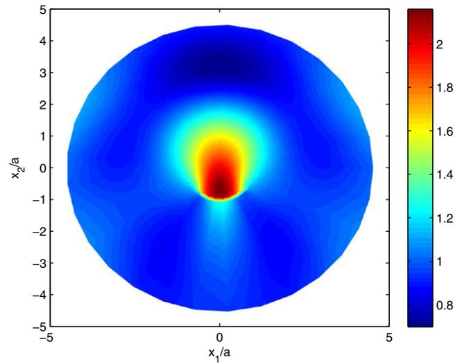
Fig. 16. L-wave scattering by a curved arch crack ( $\alpha = 45$ ): vertical displacements amplitude  $u_2/u_0$  at frequency  $\omega a/c_s = 0.8$ .
