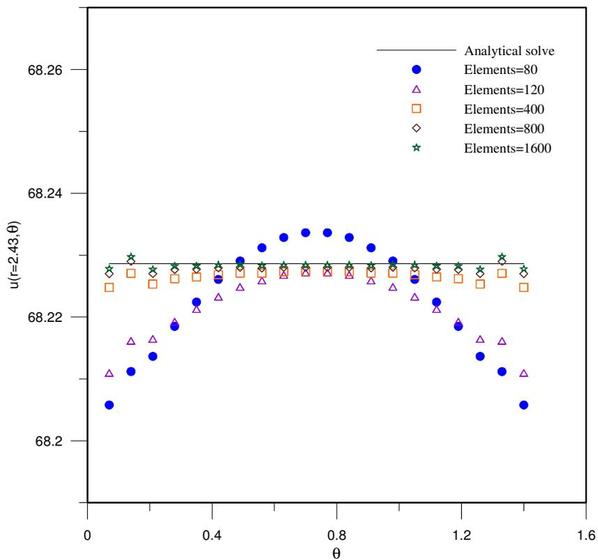
Fig. 5. The error analysis for the field solution along the radius  $r=2.43$  with the different elements.
