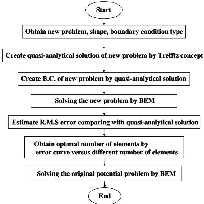
Fig. 1. Flowchart of the systematic error estimation scheme.
