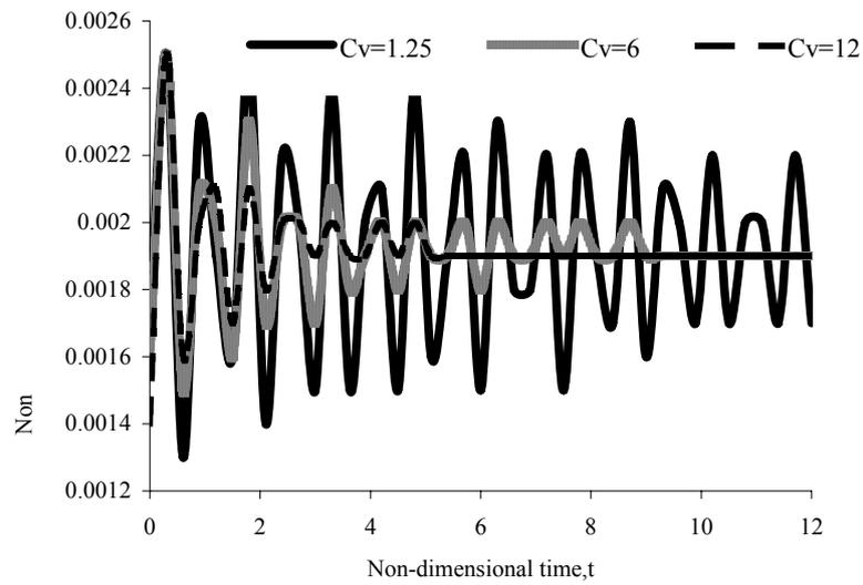
**Fig. 3:** Damped response of a simple supported pure HDPE (PCL000) square isotropic plate
