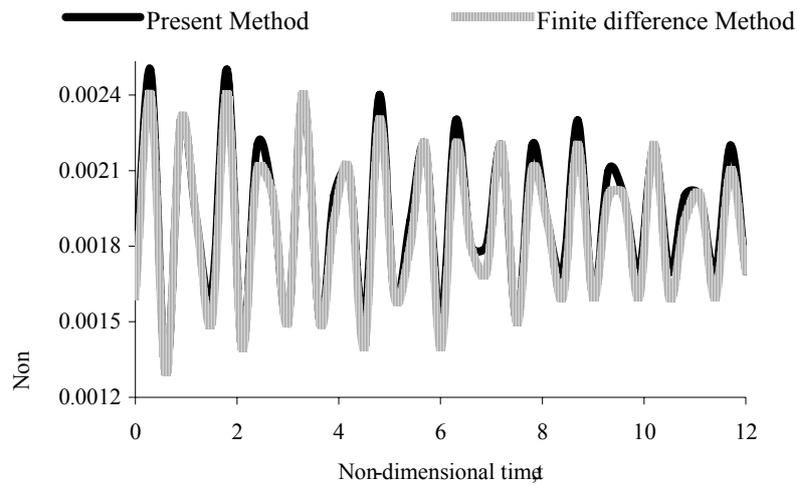
**Fig. 2:** Damped response of a simple supported pure HDPE (PCL000) square isotropic plate at damping coefficient factor  $C_v = 1.25$
