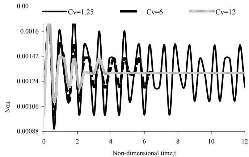
**Fig. 7:** Damped response of a simple supported treated banana fiber reinforced (PCL5T) HDPE/PCL blend square composite plate
