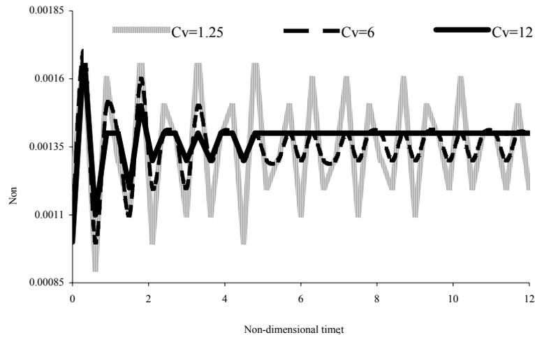
**Fig. 6:** Damped response of a simple supported untreated banana fiber reinforced (PCL5U) HDPE/PCL blend square composite plate
