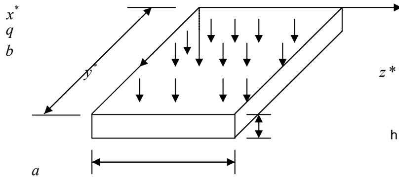
**Fig. 1:** Geometry of the banana fiber reinforced HDPE/ PCL blend composite plate
