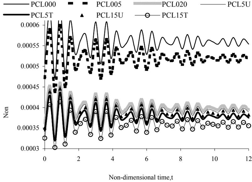
**Fig. 10:** Damped responses of a clamped edge HDPE, HDPE/PCL blends, treated and untreated banana fiber reinforced composite plate at damping coefficient factor  $C_v = 1.25$
