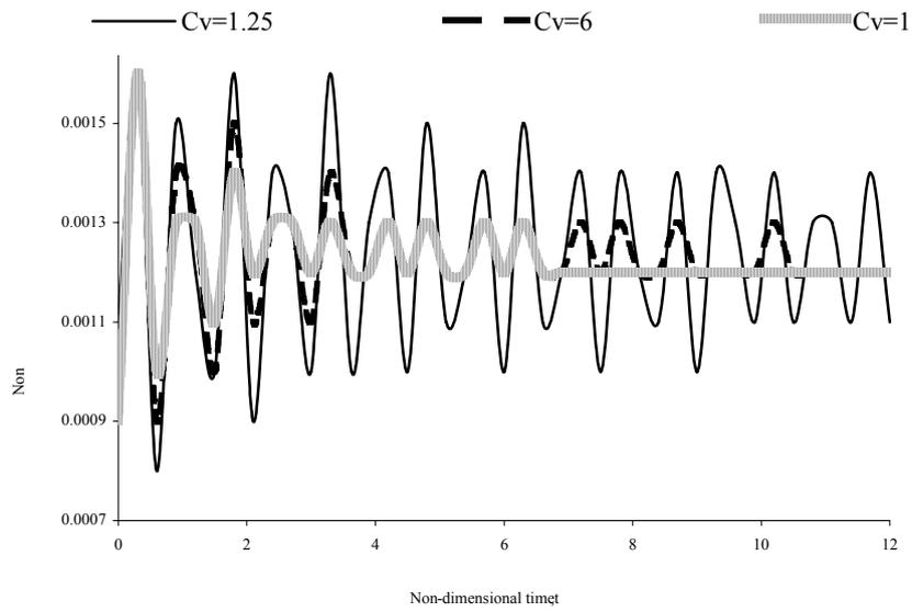
**Fig. 9:** Damped response of a simple supported treated banana fiber reinforced (PCL15T) HDPE/PCL blend square composite plate
