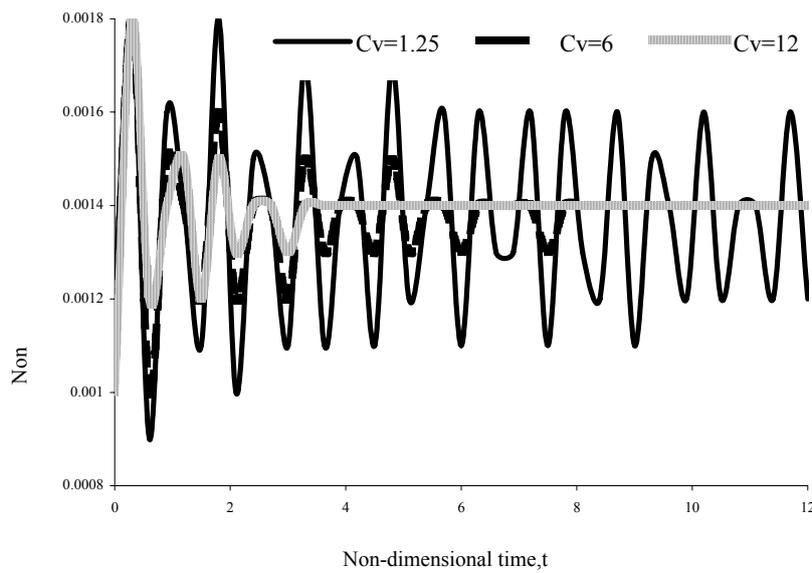
**Fig. 5:** Damped response of a simple supported HDPE/PCL blend (PCL020) square isotropic plate
