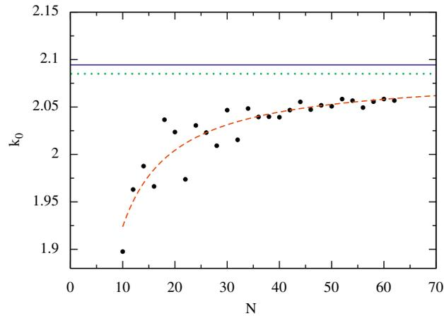
**Fig. 14.** Frequency of the fundamental mode of a spherical volume of radius  $R = 2$  with an interior spherical hole of radius  $r = \frac{1}{2}$  centered at the origin. The continuous horizontal line is the exact value  $k_0^{\text{exact}} = 2.0944$ , while the dashed curve corresponds to the fit:  $k_0^{\text{fit}}(N) = 2.08501 - 1.61284/N$ . The horizontal dotted line is the constant value  $k_0 = 2.08501$  obtained from the fit for  $N \rightarrow \infty$ .
