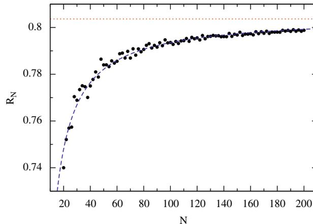
**Fig. 3.** Ratio of allowed to total points of the grid for a square membrane with a circular hole. The horizontal line is the geometric ratio, while the dashed line is the fit  $R_N^{\text{fit}} = 0.805 - 1.14/N$ .
