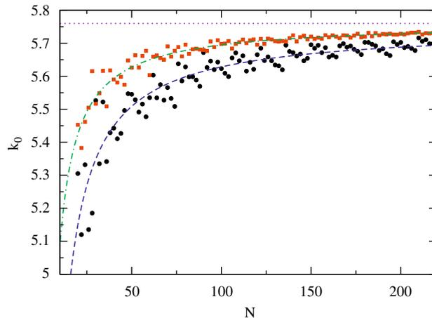
**Fig. 5.** Frequency of the fundamental mode of a hexagonal membrane with a central circular hole: the circles are obtained by orienting the membrane to have two sides parallel to the  $x$ -axis; the squares are the results obtained by performing a scale transformation in the  $y$  direction to make these two sides fall on the border of the square. The horizontal line is the result of [1], whereas the two dashed curves are fits of the two sets of data.
