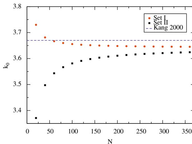
**Fig. 10.** Fundamental frequency for the square membrane of side  $\ell = 2$  with a square hole of side  $\ell_0 = 3/5\sqrt{2}$ , rotated by  $\pi/2$  with respect to the outer square. Set I (Set II) corresponds to rejecting (accepting) the points falling on the internal border. The horizontal line is the result of [15].
