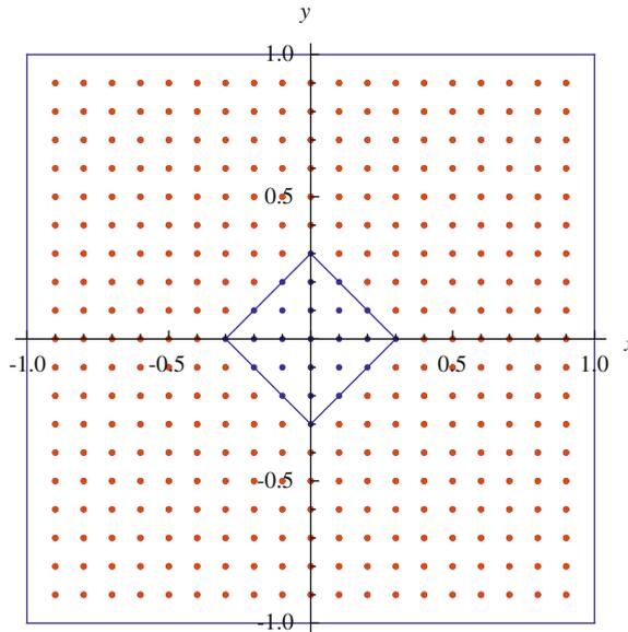
**Fig. 8.** Square membrane of side  $\ell = 2$  with a square hole of side  $\ell_0 = 3/5\sqrt{2}$ , rotated by  $\pi/2$  with respect to the outer square. The points in the figure correspond to a grid with  $N = 20$ .
