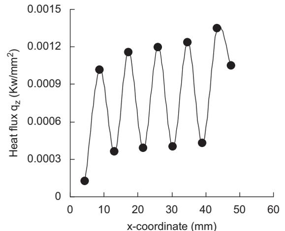
**Fig. 10.** Heat flux,  $q_z$ , along  $x$ -direction over wall and cavum of the honeycomb.
