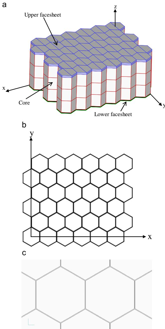
**Fig. 8.** BEM model for the honeycomb sandwich structure. (a) global model; (b) top view of the core; (c) enlarged top view of the core.
