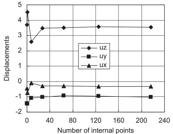
Fig. 7. Variation of displacements versus number of internal points.
