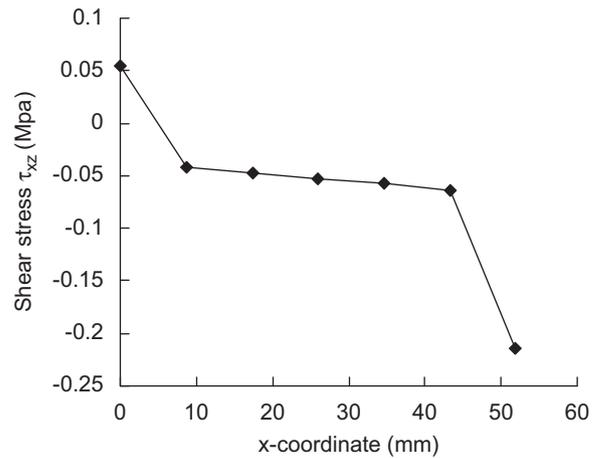
Fig. 13. Shear stress  $\sigma_{xz}$  along the  $x$ -direction.
