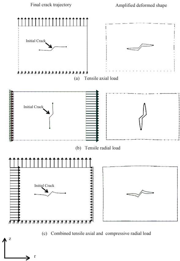
**Fig. 4.** Crack propagation of a cone crack inside a thick-walled cylinder under three different loading conditions
