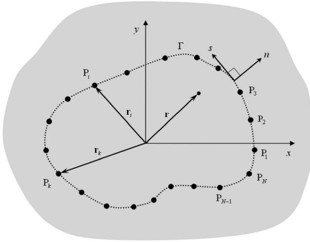
Fig. 1 An arbitrarily shaped plate depicted by the dotted contour along which  $N$  boundary nodes are distributed
