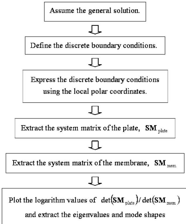
Fig. 3 Flow chart illustrating the theoretical development procedure of the present method
