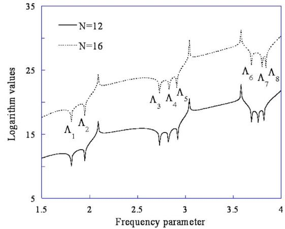
**Fig. 9** Logarithm curves for  $\det(\mathbf{SM}_{\text{plate}})/\det(\mathbf{SM}_{\text{mem}})$  of the elliptic plate when  $N=12$  and  $N=16$ ; the resolution of increment of the frequency parameter is  $1/1000$
