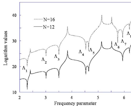
Fig. 6 Logarithm curves for  $\det(\mathbf{SM}_{\text{plate}})/\det(\mathbf{SM}_{\text{mem}})$  of the circular plate when  $N=12$  and  $N=16$ ; the resolution of increment of the frequency parameter is  $1/1000$
