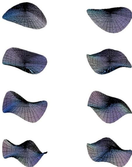
**Fig. 13 First eight mode shapes of the arbitrarily shaped plate obtained by the proposed method (N=16)**
