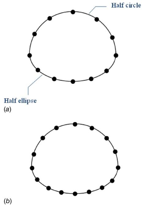
Fig. 11 Discrete boundary nodes of the arbitrarily shaped plate, composed of a half-circle and a half-ellipse, when (a)  $N=12$  and (b)  $N=16$
