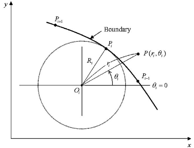
Fig. 2 Local polar coordinates system  $(r_i, \theta_i)$  for considering the free boundary condition of node  $P_i$  (the origin  $O_i$  of the coordinates system is located at the center of curvature measured at node  $P_i$  and  $R_i$  is the radius of curvature measured at node  $P_i$ )
