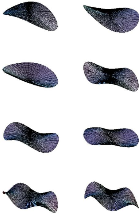
Fig. 10 First eight mode shapes of the elliptic plate obtained by the proposed method ( $N=16$ )
