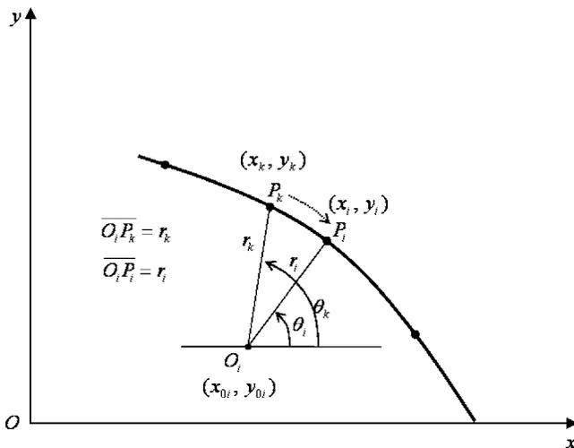
Fig. 4  $(x_i, y_i)$ ,  $(x_k, y_k)$ , and  $(x_{0i}, y_{0i})$  denote coordinates of node  $P_i$ , node  $P_k$ , and origin  $O_i$ , respectively, for the global coordinates system  $(x, y)$ ; this figure also illustrates that node  $P_k$  approaches node  $P_i$
