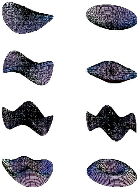
**Fig. 7 First eight mode shapes of the circular plate obtained by the proposed method ( $N=16$ )**
