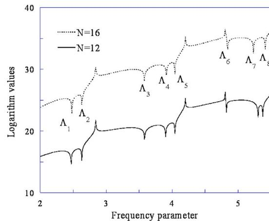
Fig. 12 Logarithm curves for  $\det(\mathbf{SM}_{\text{plate}})/\det(\mathbf{SM}_{\text{mem}})$  of the arbitrarily shaped plate when  $N=12$  and  $N=16$ ; the resolution of increment of the frequency parameter is 1/1000
