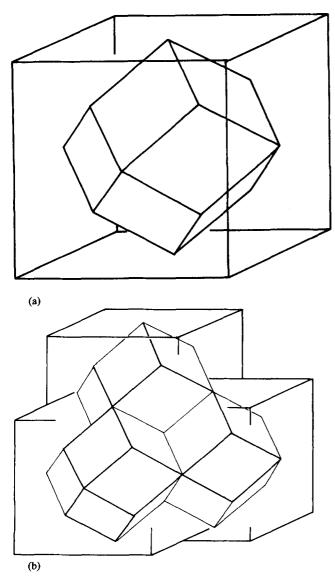
FIG. 8. Symmetric Cell. (a) Under the action of the tetrahedral group  $T_h$  the large tetrahedral domain generates a Wigner–Seitz cell (a rhombic dodecahedron) for the associated cubic *F*-lattice; (b) the Wigner–Seitz cells stack to fill all space without gaps.
