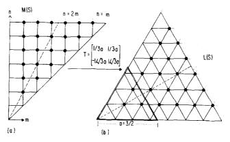
FIG. 10. *Index Sets.* (a) The standard index set, the sector **M(S)**, parametrizies the normal modes, for the  $(\pi/3|\pi/3|\pi/3)$ -triangle; (b) the natural parameter set **L(S)** is a sector with a simple relationship to the  $(\pi/3|\pi/3|\pi/3)$ -domain.
