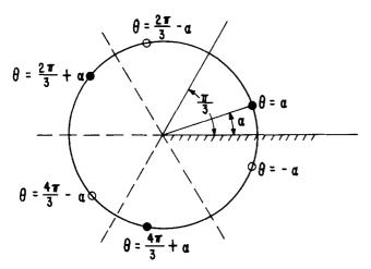
FIG. 2. The  $\pi/3$ -Wedge. The array generated is represented by dark and light circles (charges of opposite sign).
