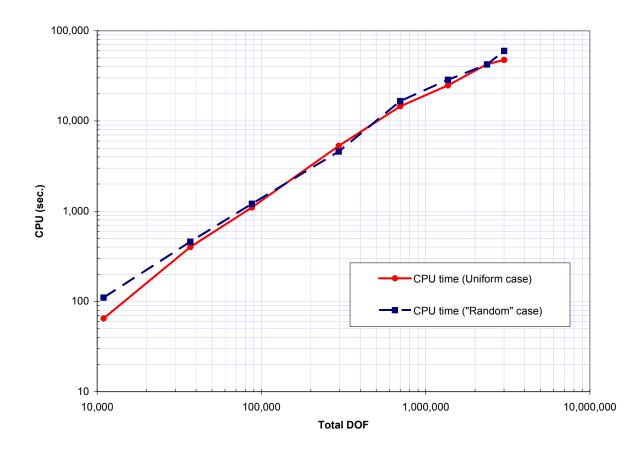
CPU time used for solving the BEM models for the short-fiber cases
