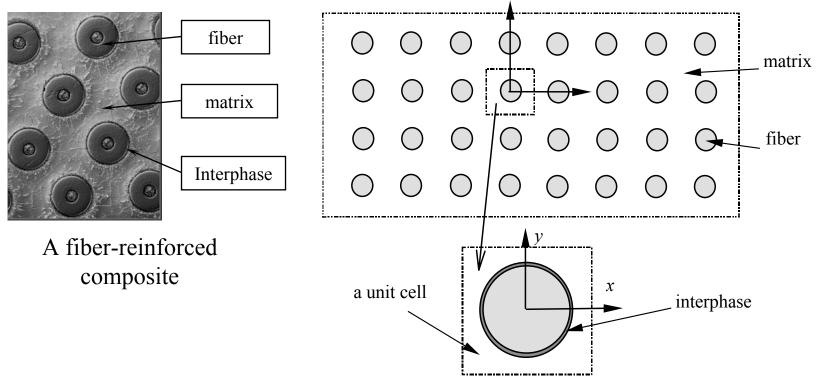
Interphases in fiber-reinforced composites are modeled using the BEM and FEM to investigate their effects on the mechanical properties and interface failures of the material.
