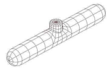
A simplified submarine model with BEM (Surface elements only)
