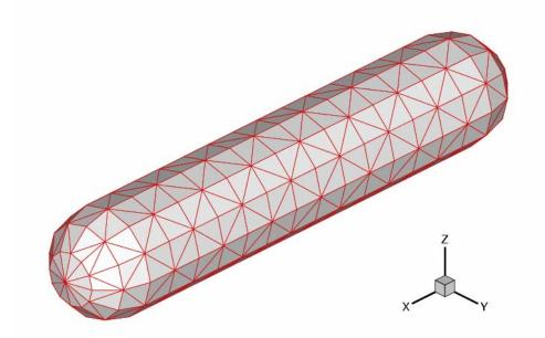
A BEM mesh used for the short fiber inclusion (with 456 constant elements)
