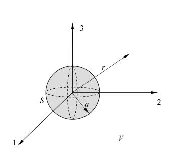
A sphere with tri-axial loading
