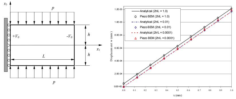
Displacement component w along the bottom edge of the strip (M = 24) for different thicknesses
