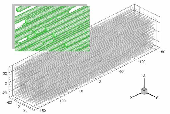
A small RVE containing 2,000 CNT fibers with the total DOF = 3,612,000 (CNT length = 50 nm, volume fraction = 10.48%). A larger model with 16,000 CNT fibers and 28.9M DOFs was solved successfully on a FUJITSU HPC2500 supercomputer (at the Kyoto University) within 34 hours. 38 CAE Research Lab
