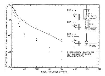
Fig. 11. Measured and theoretical field on the light-shadow boundary for a half plane with a cylindrical edge and measured field for a half plane with a rectangular edge (phase corrected for a line source).
