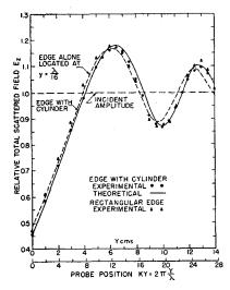
Fig. 10. Theoretical and measured diffraction from a half plane with a circular-cylindrical edge of radius=/16 and a rectangular edge of thickness=/8 (line source).
