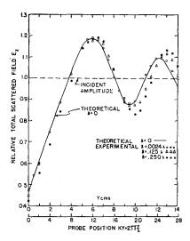
Fig. 7. Measured diffraction from a rectangular edge for different thicknesses (line source).
