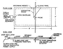
Fig. 1. Schematic layout of parallel-plate region and microwave components.
