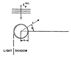
Fig. 8. Coordinate system for scattering from a half plane with a cylindrical edge (line source).
