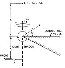
Fig. 3. Coordinate system for scattering from a wedge.
