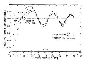
Fig. 6. Approximate theoretical and measured diffraction patterns from 45 and 90 wedges (line source).
