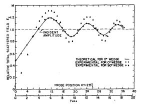
Fig. 5. Measured diffraction patterns from 0° and 90° wedges (line source).
