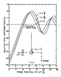
Fig. 9. Theoretical diffraction pattern from a half plane with a cylindrical edge (phase corrected for a line source).
