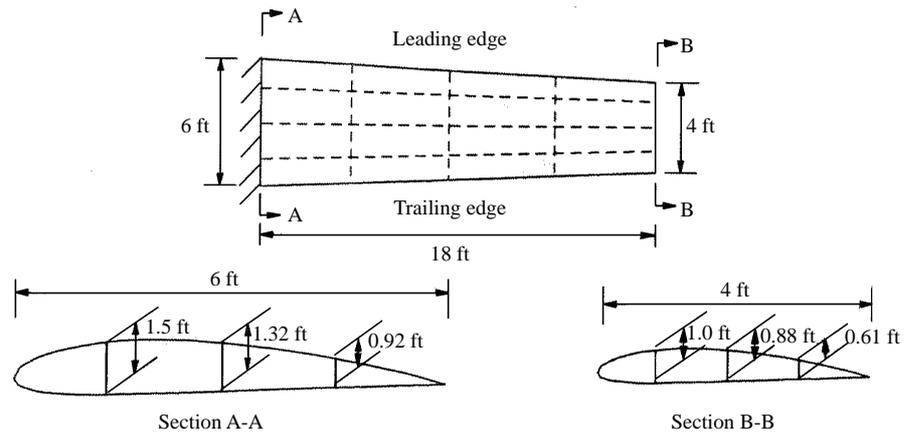
(a) Geometry of a composite wing
