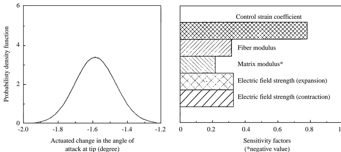
Fig. 5 Probability density function of actuated change in the angle of attack and sensitivity factors at 0.999 probability
