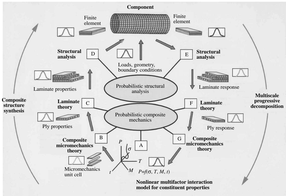
Fig. 3 Concept of probabilistic assessment of composite structures
