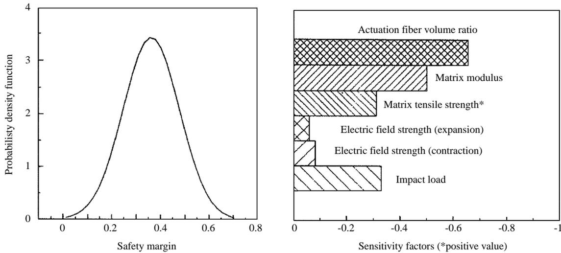
Fig. 8 Probability density function of safety margin and sensitivity factors at safety margin equal to zero
