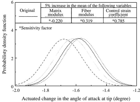
Fig. 6 Probability density function of actuated change in the angle of attack with 5% increase in the mean of one random variable
