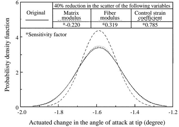
Fig. 7 Probability density function of actuated change in the angle of attack with 40% reduction in the scatter of one random variable
