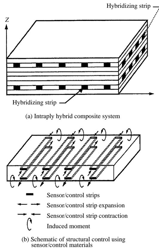
Fig. 2 Adaptation of intraply hybrid to smart composite system
