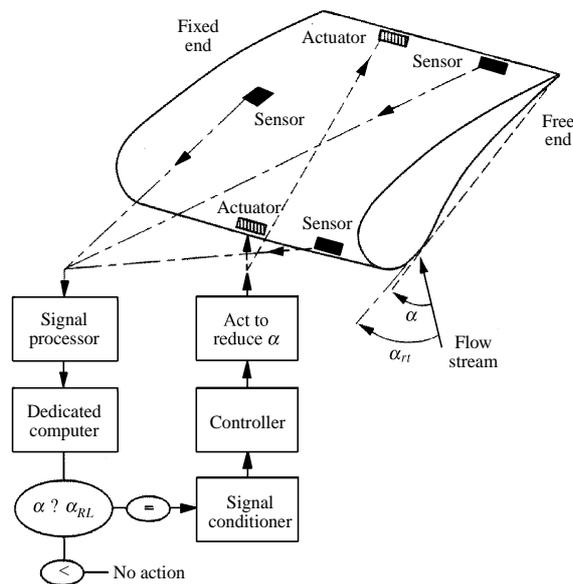
Fig. 1 Conceptual diagram of smart composite aircraft wing system
