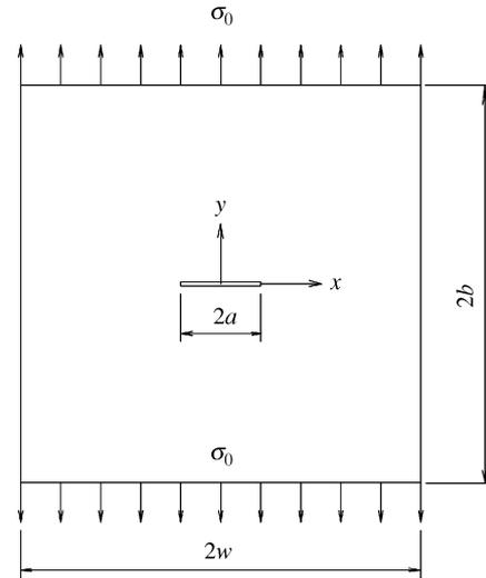
Fig. 1 The finite cracked body
