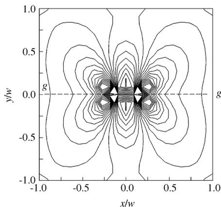
Fig. 4 Contours of strain energy density with  $b/w=1$
