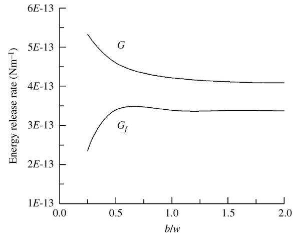
Fig. 8 Energy release rate of aluminum alloy
