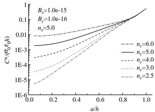
Fig. 7 Influence of creep index  $n$  on the  $C^*$
