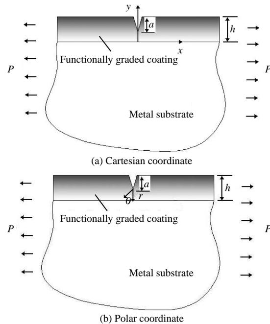
Fig.1 Coating and substrate system
