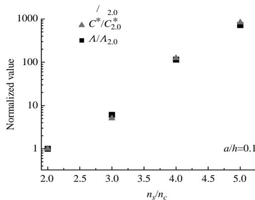
Fig. 11 Normalized value of  $C^*$  and  $\Lambda$  at different creep index ratios
