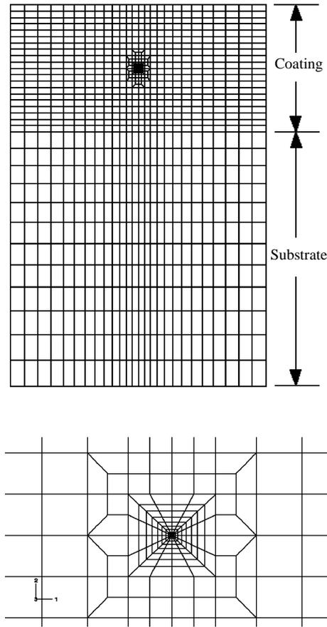
Fig. 2 Entire mesh and detail mesh at the crack tip
