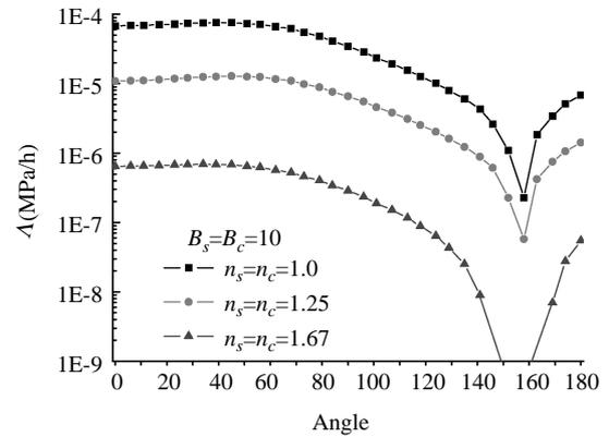
Fig. 9 Influence of creep index  $n$  on strain energy density rate factor
