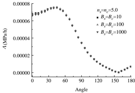
Fig. 8 Influence of creep coefficient  $B$  on strain energy density rate factor
