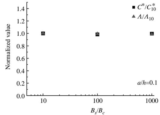
Fig. 10 Normalized value of  $C^*$  and  $\Lambda$  at different creep coefficient ratios
