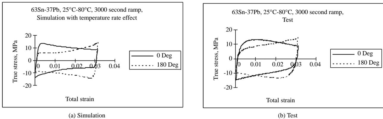
Fig. 3 In-phase and Out-of-phase TMF hysteresis loops for 63Sn-37Pb solder at strain rate of  $10^{-5}/s$
