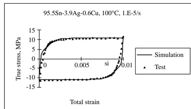
Fig. 5 Isothermal hysteresis loops for 95.5Sn-3.9Ag-0.6Cu solder under 100°C at strain rate of  $10^{-5}/s$
