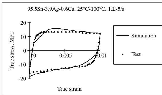
Fig. 6 In-phase TMF hysteresis loops for 95.5Sn-3.9Ag-0.6Cu solder under the temperature range from 25°C to 100°C at strain rate of  $10^{-5}$ /s
