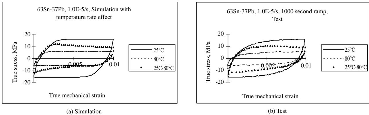
Fig. 2 Isothermal and TMF hysteresis loops for 63Sn-37Pb solder at strain rate of  $10^{-5}/s$
