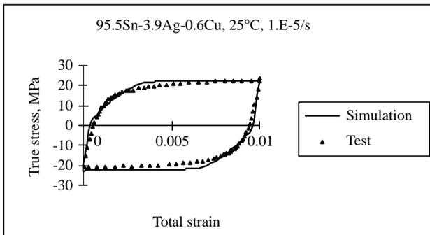
Fig. 4 Isothermal hysteresis loops for 95.5Sn-3.9Ag-0.6Cu solder under 25°C at strain rate of  $10^{-5}/s$
