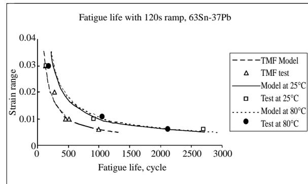
Fig. 7 Isothermal and TMF fatigue life for 63Sn-37Pb solder
