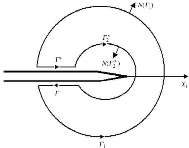
Fig. 2  $J$ -integral contour around crack tip
