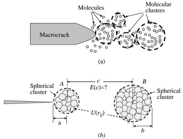
Fig. 1. (a) Molecular clusters (lattices) in the immediate vicinity of a crack tip. (b) Molecules contained in each cluster and the cluster potential  $E(d)$ , where  $d$  is the central distance between two adjacent clusters.
