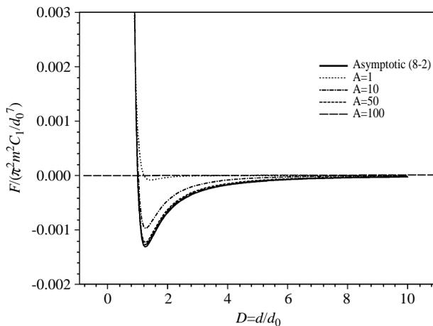
Fig. 4. Comparison of the interaction forces – The asymptotic expression, Eq. (20) with identical spheres (the 8-2 relation), and the full expression, Eq. (14),  $A=a/d_0$ .
