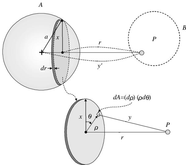
Fig. 2. Potential between a representative molecule P in sphere B and sphere A – The Coordinate system.
