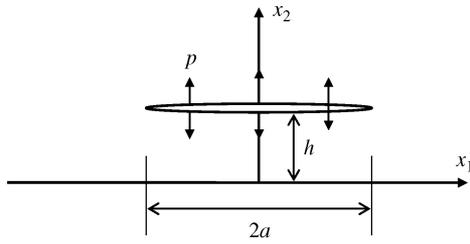
Fig. 3 An internal horizontal crack under a uniform pressure  $p$  in a half-plane
