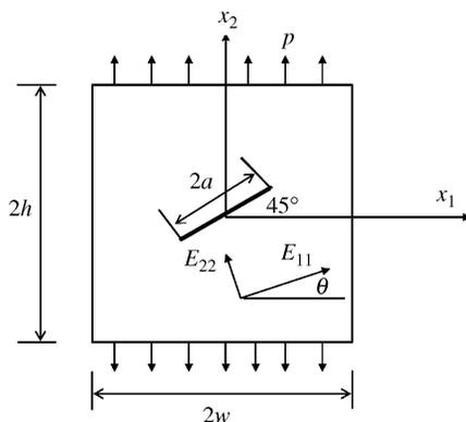
Fig. 5 An inclined crack in a finite plate under a uniform tension  $p$
