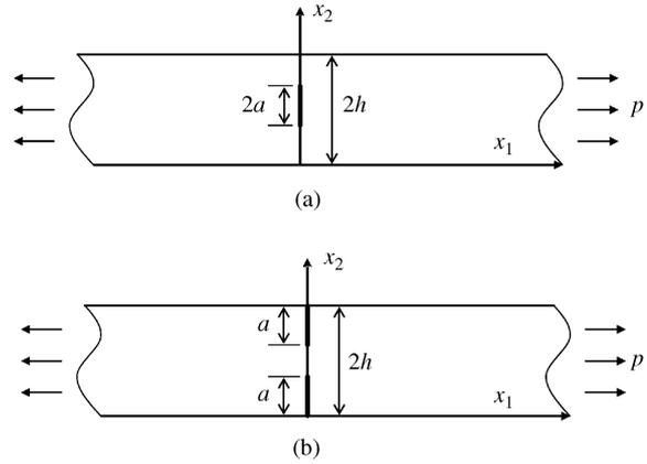
Fig. 4 (a) An internal crack, (b) double edge cracks in a strip under a uniaxial tension  $p$
