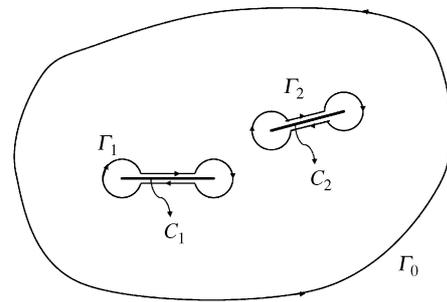
Fig. 1 A body bounded by an external boundary  $\Gamma_0$  containing  $N=2$  crack lines
