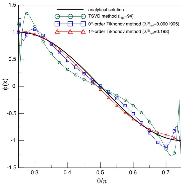
**Fig. 6** Numerical results by employing the TSVD method, the zero and first order Tikhonov methods, respectively, and using 200 nodes for the case 1
