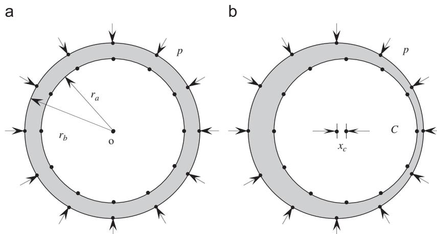
Fig. 5. A thin coating with nonuniform thickness on a shaft.
