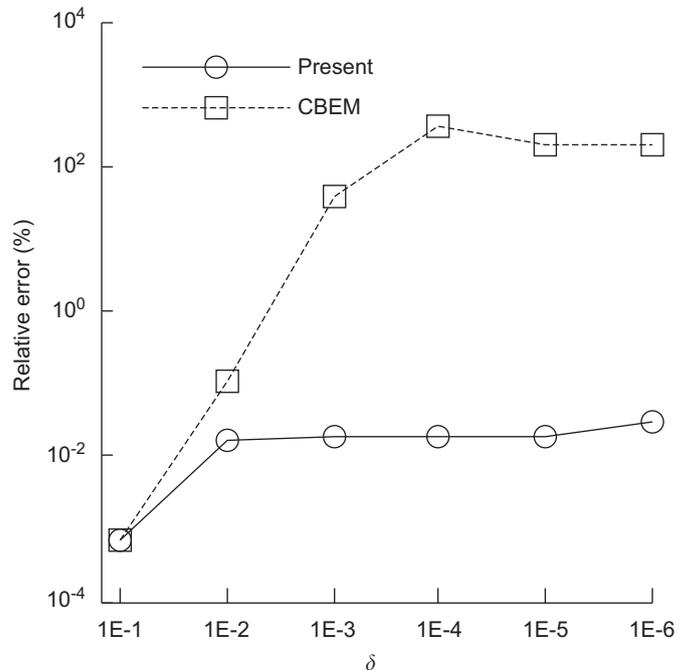
Fig. 3. Relative errors (%) of the tangential stresses  $\sigma_\theta$  at the boundary node  $A$ .
