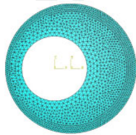
FEM mesh (No. of nodes=1,734 No. of elements=3,218)
