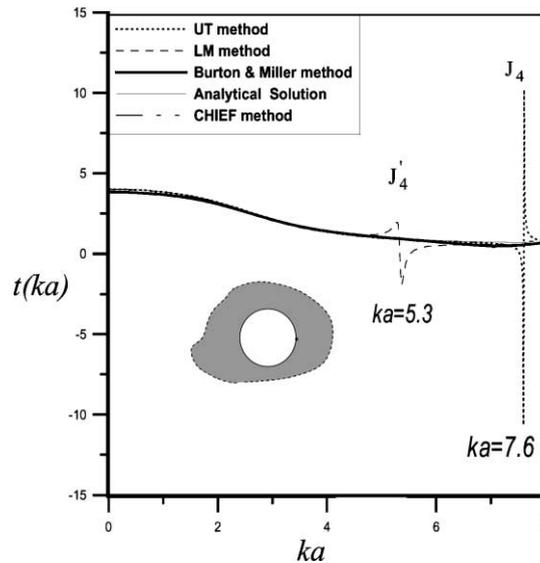
Fig. 3. The positions of irregular values using different methods.
