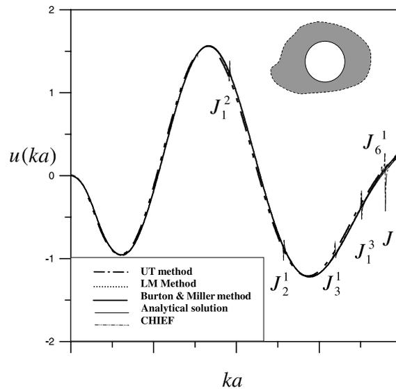
Fig. 12. The positions of irregular values using different methods.
