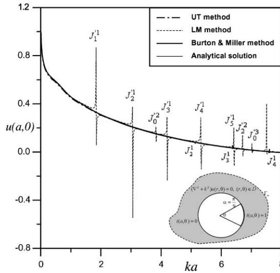
Fig. 6. The positions of irregular values using different methods.
