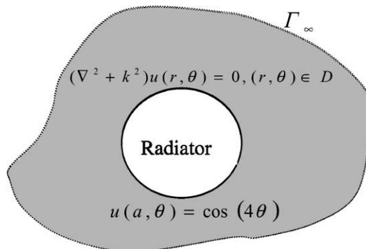
**Fig. 1.** The uniform radiation problem (Dirichlet condition) for a cylinder.
