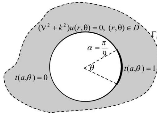
Fig. 4. The nonuniform radiation problem (Neumann condition) for a cylinder.
