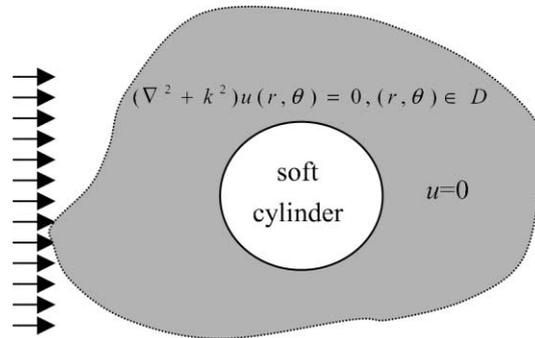
Fig. 7. The scattering problem (Dirichlet condition) for a cylinder.
