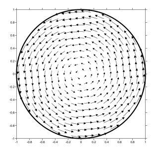
Figure 2. Stress field of the circular case
