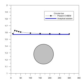
Figure 1. Torsional rigidity versus the number of elements in circular case
