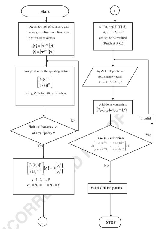
Fig. 1. The flowchart of a criterion to check the validity of the selected CHIEF point.
