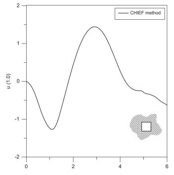
**Fig. 15.** The boundary value versus the wave number k by locating two CHIEF points away from the nodal line.
