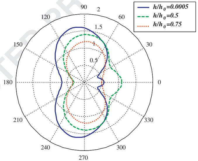
Fig. 6. DMCF along the circular boundary of a flexible inclusion at different thicknesses, solid line for  $h/h_0=0.0005$ , dashed line for  $h/h_0=0.5$  and dotted line for  $h/h_0=0.75$  ( $ka=3.0$ ).
