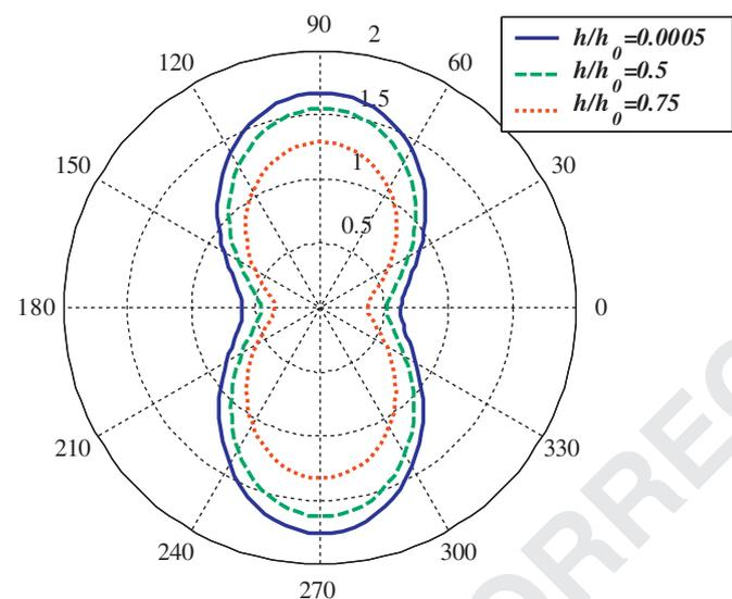
Fig. 20. DMCF along the circular boundary of the upper flexible inclusion at different thicknesses, solid line for  $h/h_0=0.0005$ , dashed line for  $h/h_0=0.5$  and dotted line for  $h/h_0=0.75$  ( $ka=0.5$  and  $L/a=4.0$ ).
