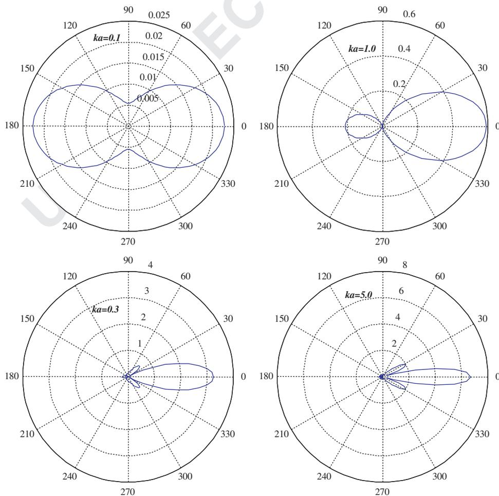
**Fig. 19.** Far-field scattering pattern for two flexible inclusions with  $h/h_0=0.7$  and  $L/a=2.1$  at various dimensionless wave numbers  $ka=0.1, 1.0, 3.0$  and  $5.0$ .
