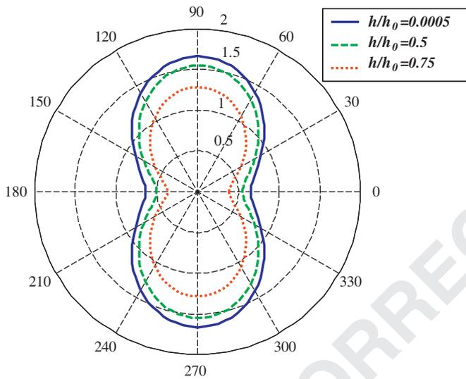
Fig. 4. DMCF along the circular boundary of a flexible inclusion at different thicknesses, solid line for  $h/h_0=0.0005$ , dashed line for  $h/h_0=0.5$  and dotted line for  $h/h_0=0.75$  ( $ka=0.5$ ).
