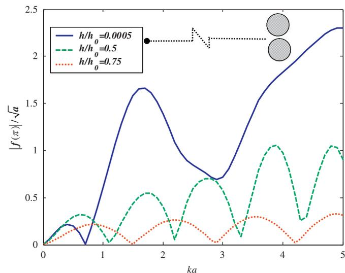
**Fig. 18.** Far-field backscattering amplitude versus the dimensionless wave number at different thicknesses of a flexible inclusion, solid line for  $h/h_0=0.0005$ , dashed line for  $h/h_0=0.5$  and dotted line for  $h/h_0=0.75$  ( $L/a=2.1$ ).
