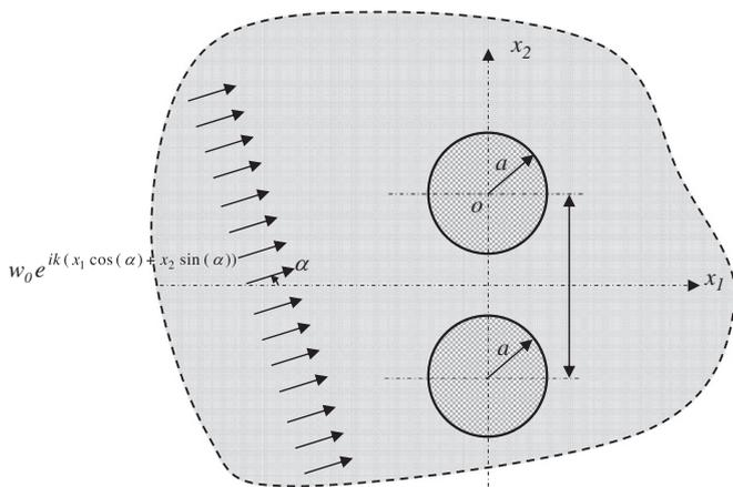
Fig. 10. An infinite thin plate with two circular inclusions subject to an incident flexural wave with an incident angle  $\alpha$
