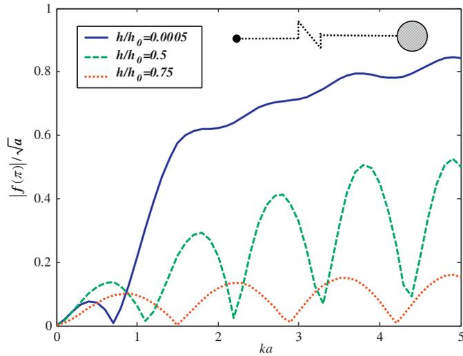
Fig. 8. Far-field backscattering amplitude versus the dimensionless wave number at different thicknesses of a flexible inclusion, solid line for  $h/h_0=0.0005$ , dashed line for  $h/h_0=0.5$  and dotted line for  $h/h_0=0.75$ .
