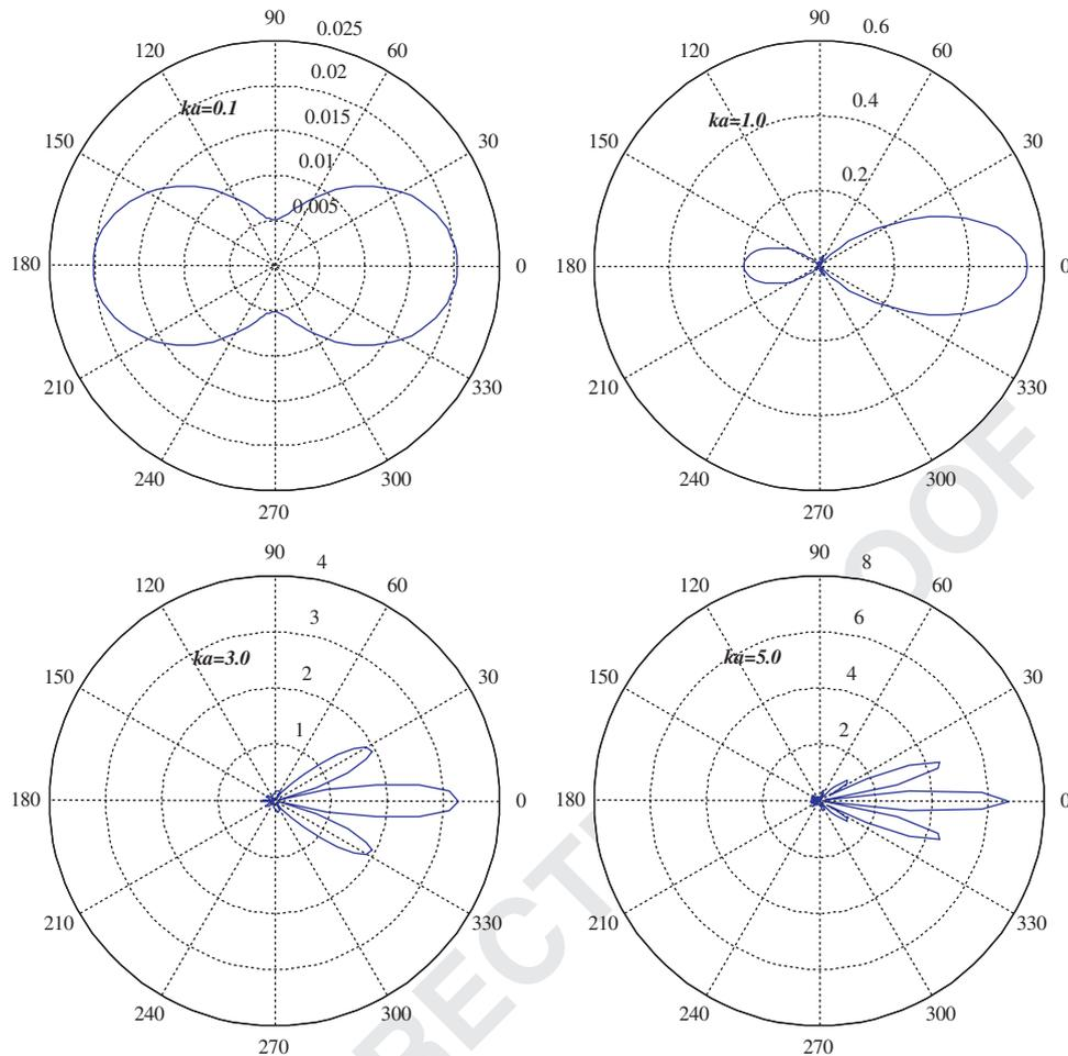
Fig. 24. Far-field scattering pattern for two flexible inclusions with  $h/h_0=0.7$  and  $L/a=4.0$  at various dimensionless wave numbers  $ka=0.1, 1.0, 3.0$  and  $5.0$ .
