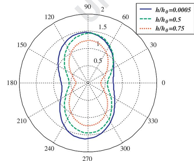
Fig. 21. DMCF along the circular boundary of the upper flexible inclusion at different thicknesses, solid line for  $h/h_0=0.0005$ , dashed line for  $h/h_0=0.5$  and dotted line for  $h/h_0=0.75$  ( $ka=1.0$  and  $L/a=4.0$ ).
