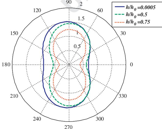
Fig. 5. DMCF along the circular boundary of a flexible inclusion at different thicknesses, solid line for  $h/h_0=0.0005$ , dashed line for  $h/h_0=0.5$  and dotted line for  $h/h_0=0.75$  ( $ka=1.0$ ).
