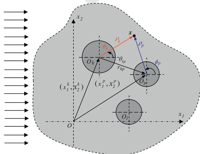
Fig. 1. Problem statement for an infinite thin plate with multiple circular inclusions subject to an incident flexural wave.
