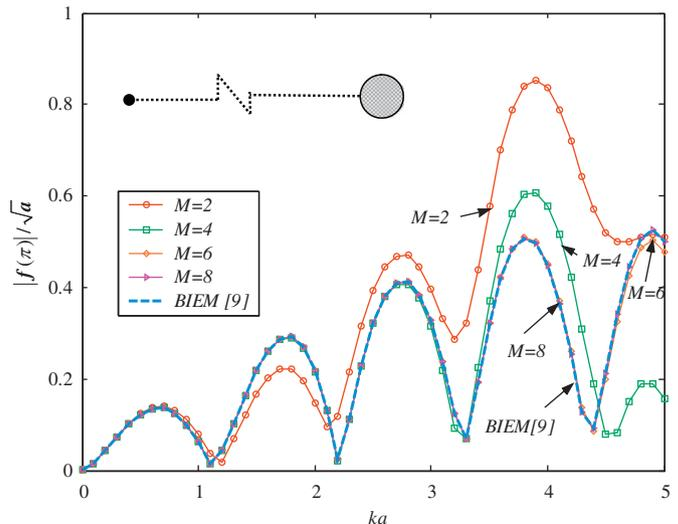
Fig. 7. Far-field backscattering amplitude versus the dimensionless wave number by using different number of coefficients.
