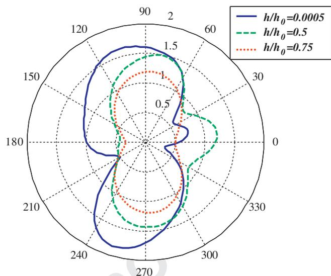
Fig. 22. DMCF along the circular boundary of the upper flexible inclusion at different thicknesses, solid line for  $h/h_0=0.0005$ , dashed line for  $h/h_0=0.5$  and dotted line for  $h/h_0=0.75$  ( $ka=3.0$  and  $L/a=4.0$ ).
