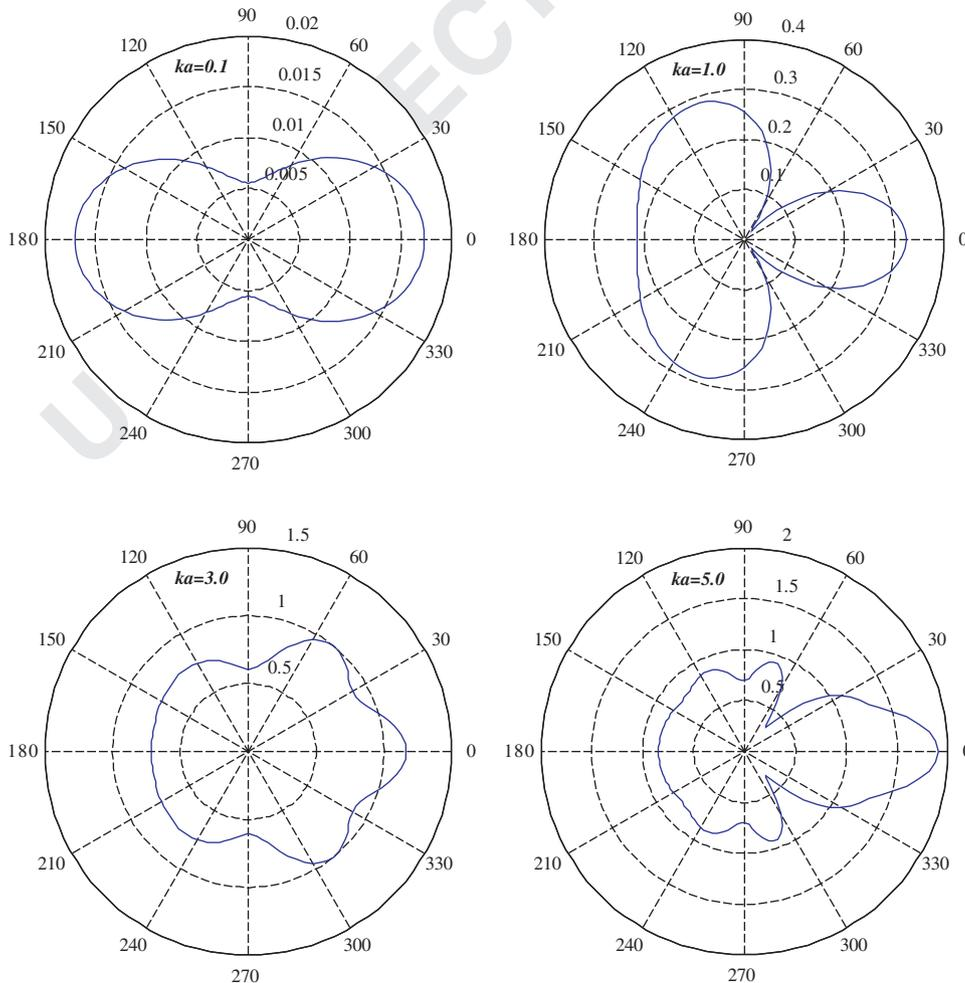
Fig. 9. Far-field scattering pattern for a flexible inclusion with  $h/h_0=0.0005$  at various dimensionless wave numbers  $ka=0.1, 1.0, 3.0$  and  $5.0$ .
