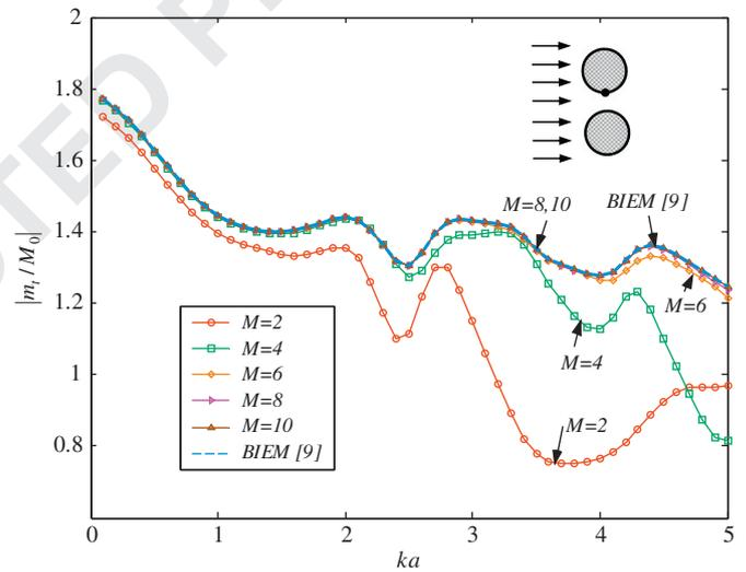
Fig. 12. DMCF on the upper circular boundary ( $\theta = -\pi/2$ ) versus the dimensionless wave number by using different number of coefficients ( $L/a=4.0$ ).
