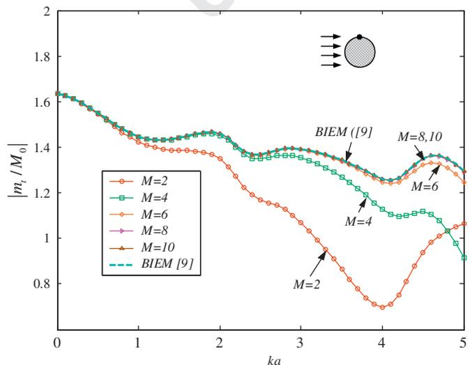
Fig. 2. DMCF on the circular boundary ( $\theta = \pi/2$ ) versus the dimensionless wave number by using different number of coefficients.
