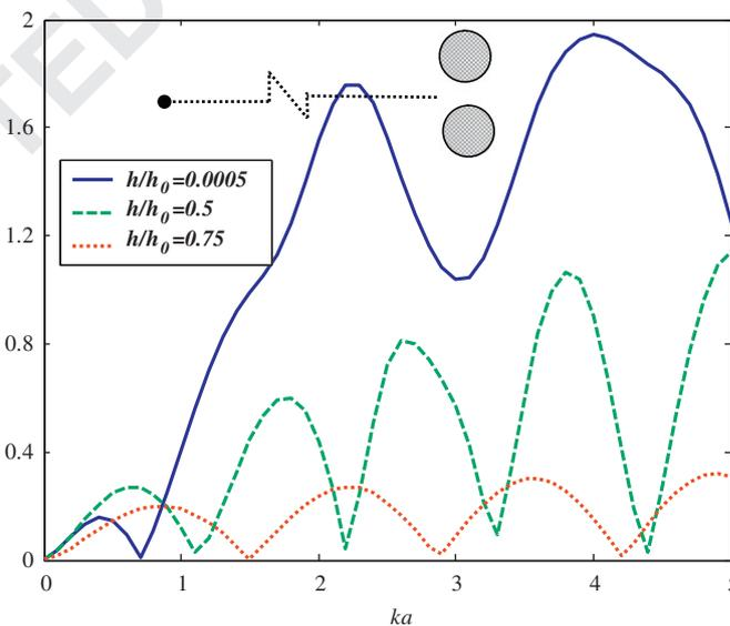
Fig. 23. Far-field backscattering amplitude versus the dimensionless wave number at different thicknesses of a flexible inclusion, solid line for  $h/h_0=0.0005$ , dashed line for  $h/h_0=0.5$  and dotted line for  $h/h_0=0.75$  ( $L/a=4.0$ ).
