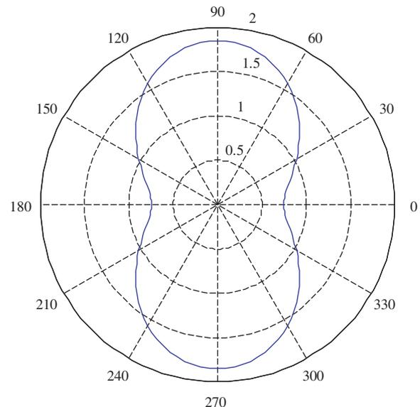
Fig. 3. DMCF along the circular boundary of a flexible inclusion in an infinite plate ( $ka=0.005$  and  $h/h_0=0.0005$ ).
