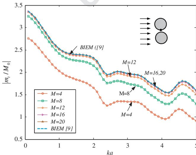
Fig. 11. DMCF on the upper circular boundary ( $\theta = -\pi/2$ ) versus the dimensionless wave number by using different number of coefficients ( $L/a=2.1$ ).
