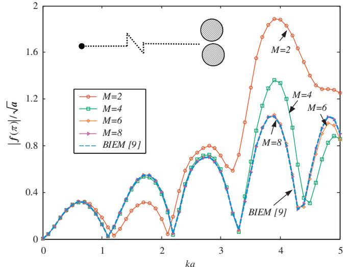
Fig. 13. Far-field backscattering amplitude versus the dimensionless wave number by using different number of coefficients ( $L/a=2.1$ ).
