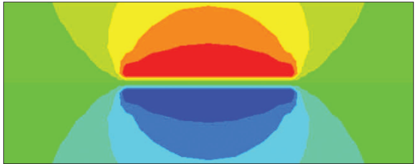
10. The results of electric potential field (equipotential lines) of the parallel-plate capacitor using FEM (red: +V_0 ; blue: -V_0 ).
