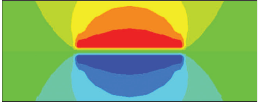
9. The results of electric potential field (equipotential lines) of the parallel-plate capacitor using DBEM (red: +V_0 ; blue: -V_0 ).
