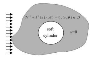
Fig. 7. The scattering problem (Dirichlet condition) for a cylinder.
