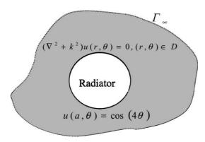
Fig. 1. The uniform radiation problem (Dirichlet condition) for a cylinder.
