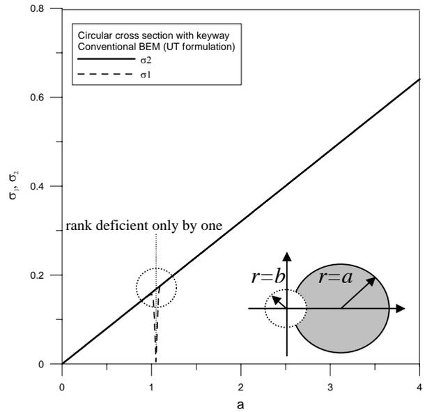
Fig. 3 (b) The second minimum singular value versus scale using the conventional BEM (UT formulation).
