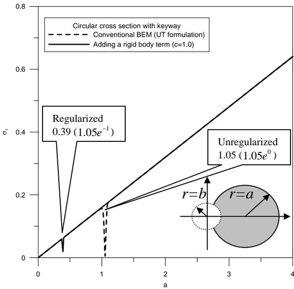
Fig. 3 (a) The first minimum singular value versus scale using the conventional BEM (UT formulation) and method of adding a rigid body term.
