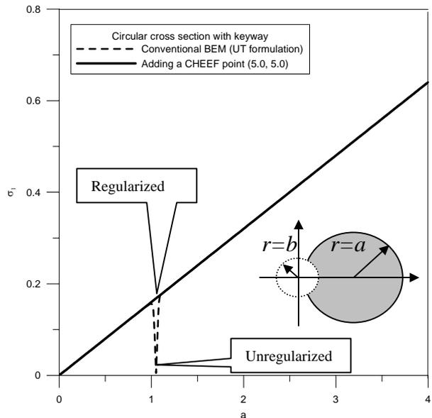
Fig. 3 (d) The first minimum singular value versus scale by using the conventional BEM (UT formulation) and CHEEF method.
