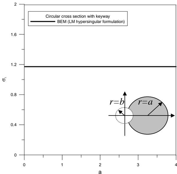
Fig. 3 (c) The first minimum singular value versus scale by using the hypersingular equation (LM formulation).
